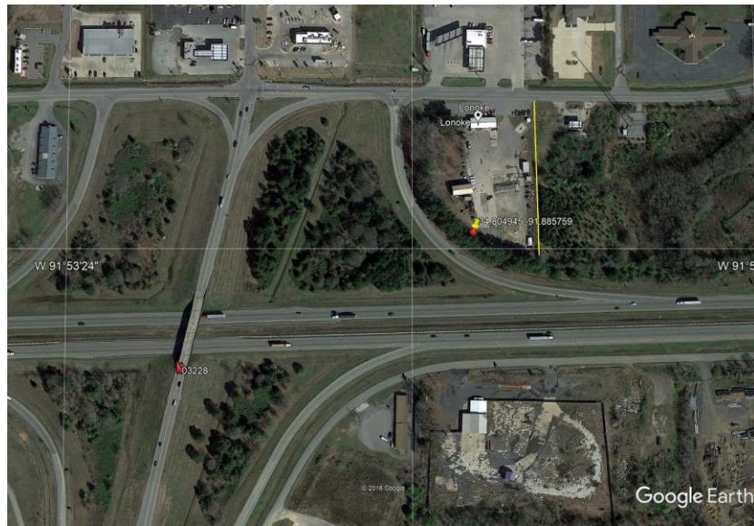
Figure A-26. The Location of ReMi and MASW Lines is Highlighted in Yellow for Site 7
