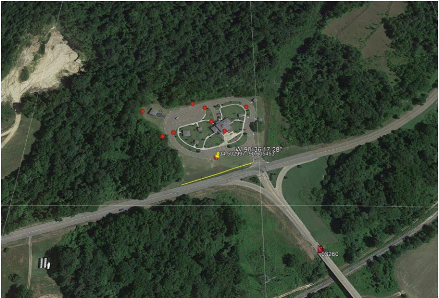
Figure A-18. The Location of ReMi and MASW Lines is Highlighted in Yellow for Site 5
