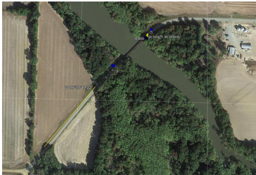
Figure A-10. The Location of ReMi and MASW Lines is Highlighted in Yellow for Site 3
