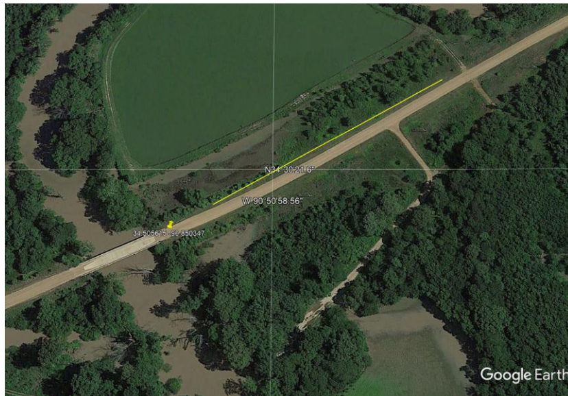
Figure A-14. The Location of ReMi and MASW Lines is Highlighted in Yellow for Site 4
