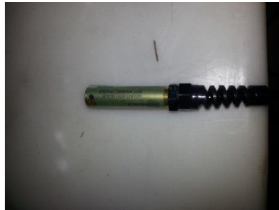
Figure 17. Data Transfer Cable from Geode to Geode, or from Geode to Software Console on Laptop
