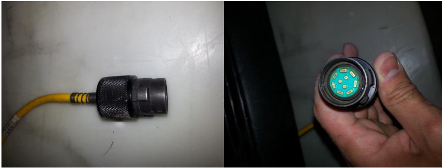
Figure 17. Data Transfer Cable from Geode to Geode, or from Geode to Software Console on Laptop
