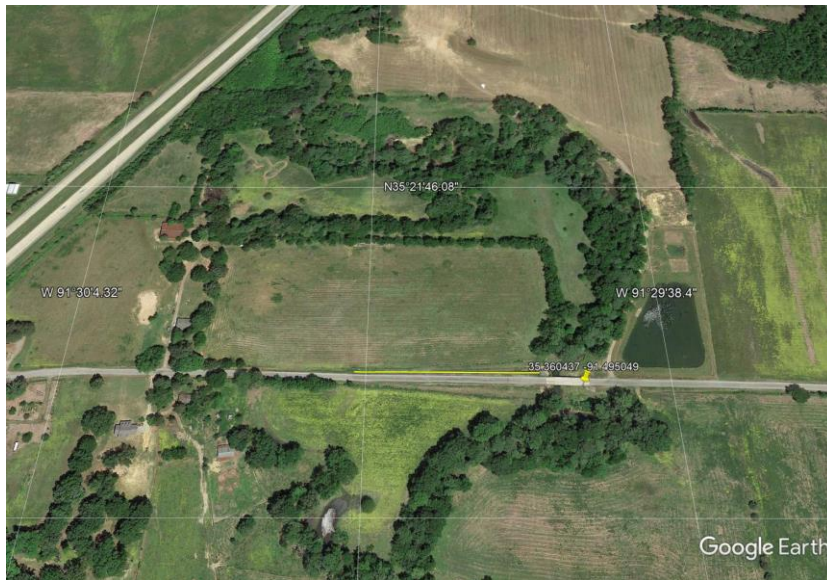
Figure A-34. The Location of ReMi and MASW Lines is Highlighted in Yellow for Site 9
