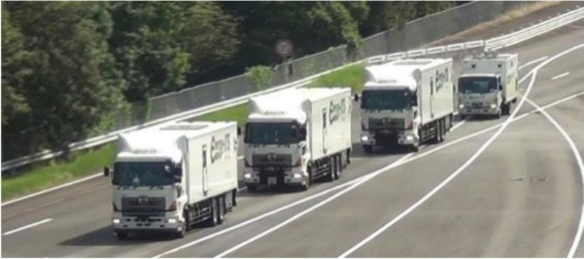
Figure 3. Photo. Truck platoon in Energy ITS project.
