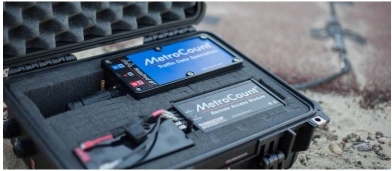
The RidePod® BT can be extended with FieldPod® remote access in a range of customisable enclosures like the pictured Pelican case.
