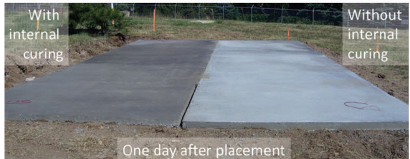
Figure 1. Comparison between concrete slabs poured with and without internal curing in field conditions
