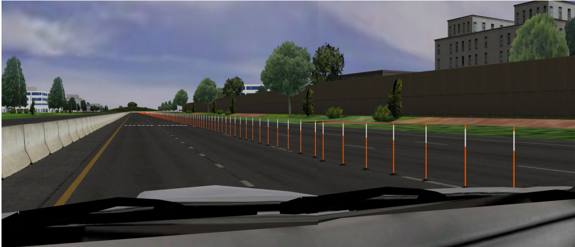
Figure 3-5: Orange Delineators with White Reflective Sheet and Asphalt Surface
