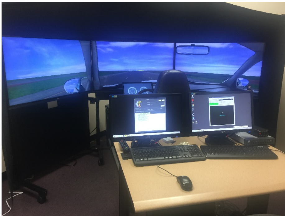
Figure 3-1: UCF Driving Simulator
