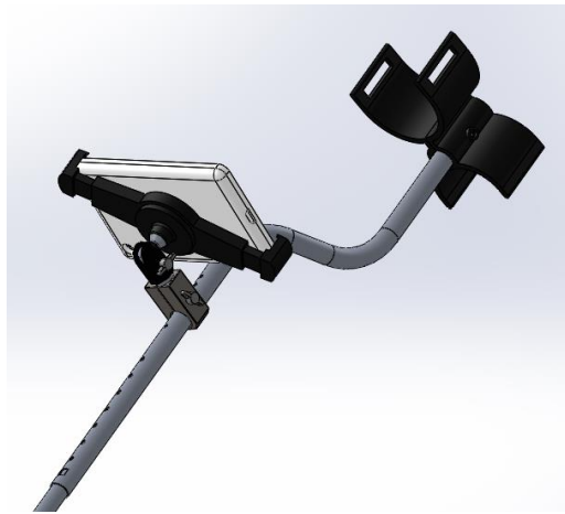
Figure 16: CIS handle. iPad is attached via a tripod clamped to the handle. Arm holder at the top of the handle helps to keep the CIS steady.
