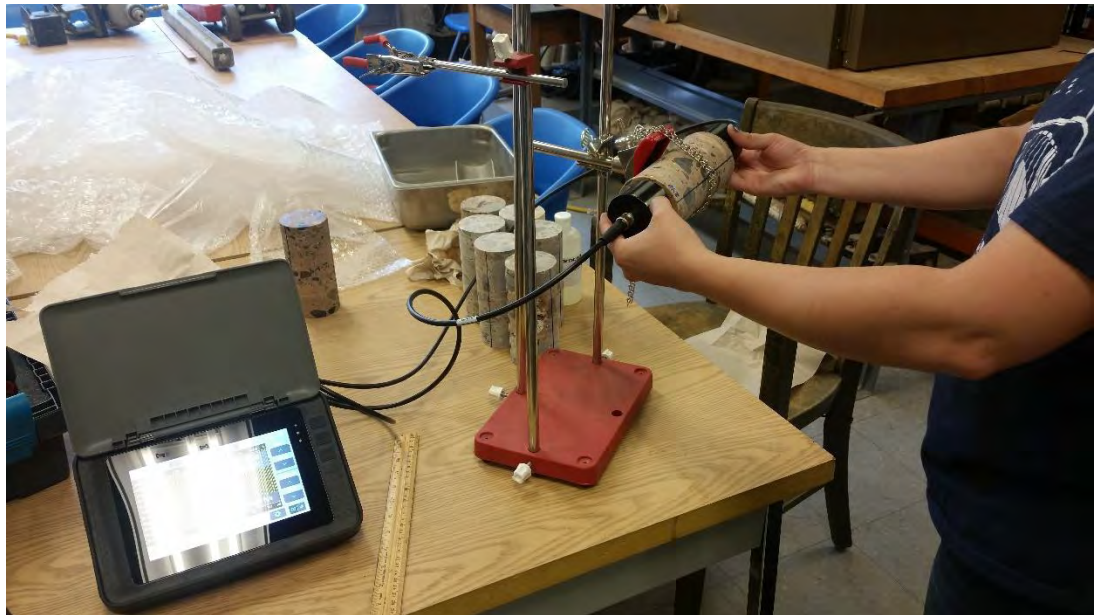
Figure 3.12: Ultrasonic testing configuration.
