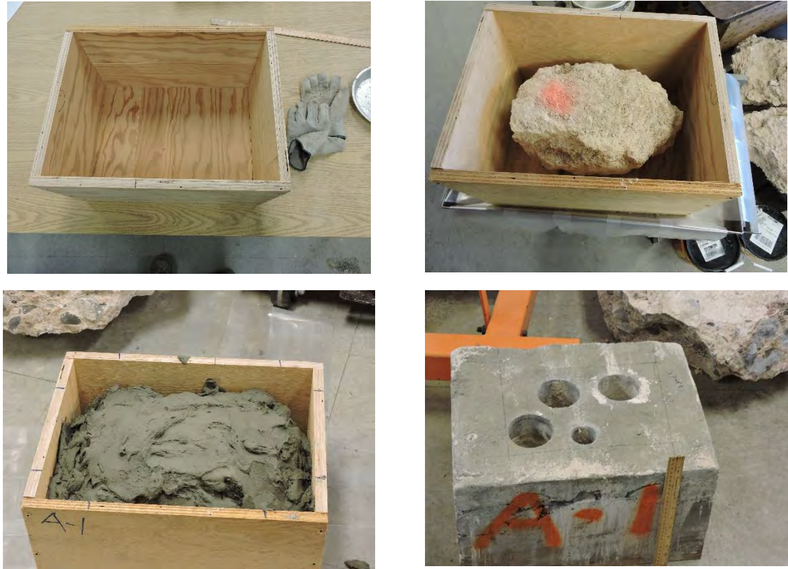
Figure 3.10: Stages of constructing the sample confined in grout.
