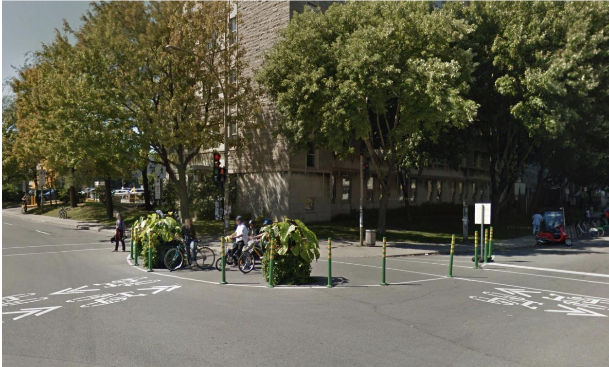
Figure 4.13 Montreal Protected Intersection (Source: Alta Planning + Design, 2015)
