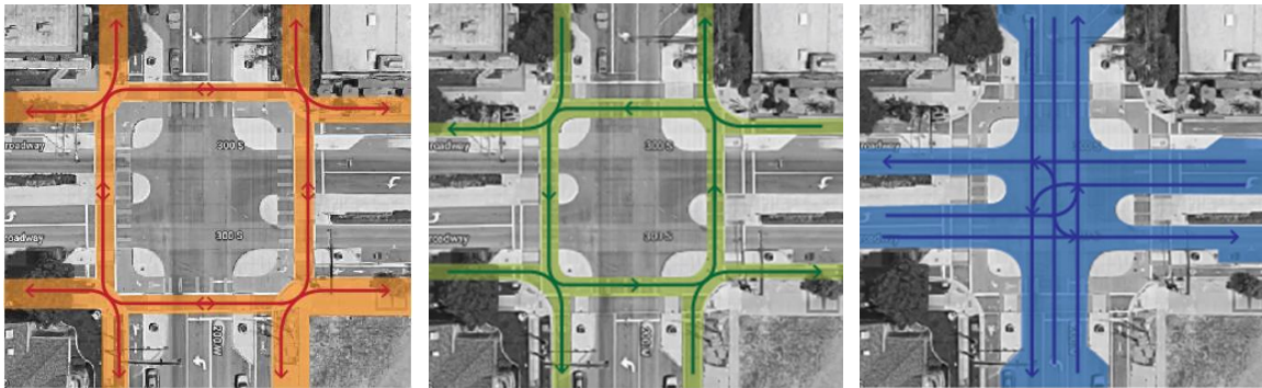
Figure 4.16 Salt Lake City Protected Intersection: Travel Modes Separation
