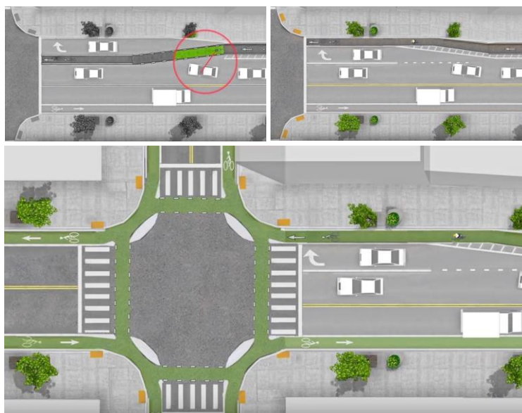
Figure 4.4 Dutch Bike Intersection Design Development (Source: Wagenbuur, 2011)
