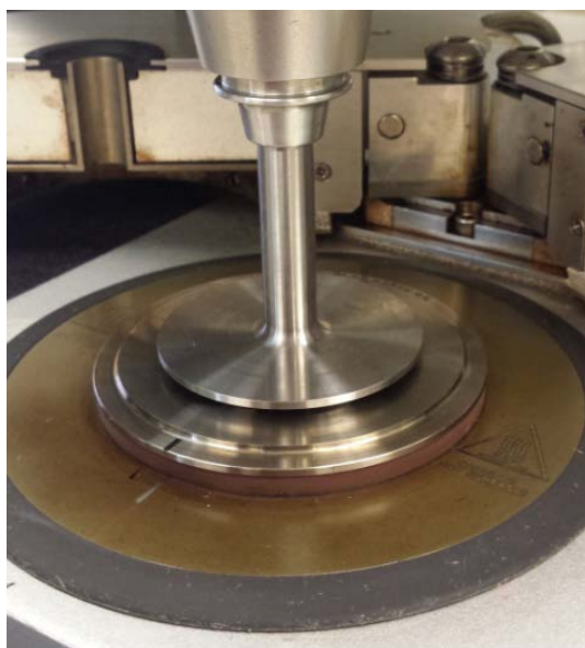
Figure 2. Dynamic Viscosity Measurement with 50 mm Plate.
