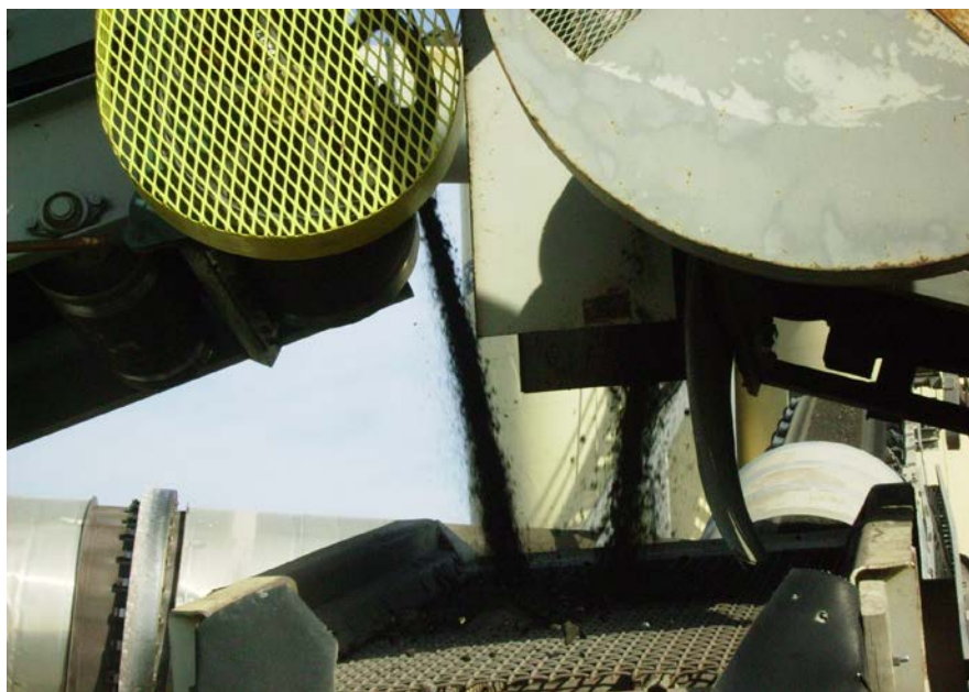
Figure 15. Vibratory Scalping Screen (after Morton, 2011).
