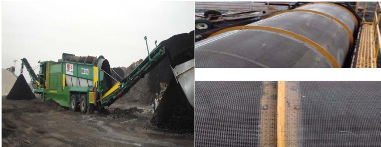
Figure 6. Screening RAS Using Trommel Screen Machine.
