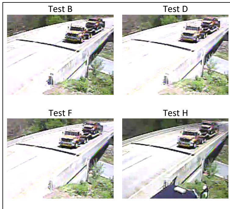
Figure 3.12: Passages of test truck over fast lane.
