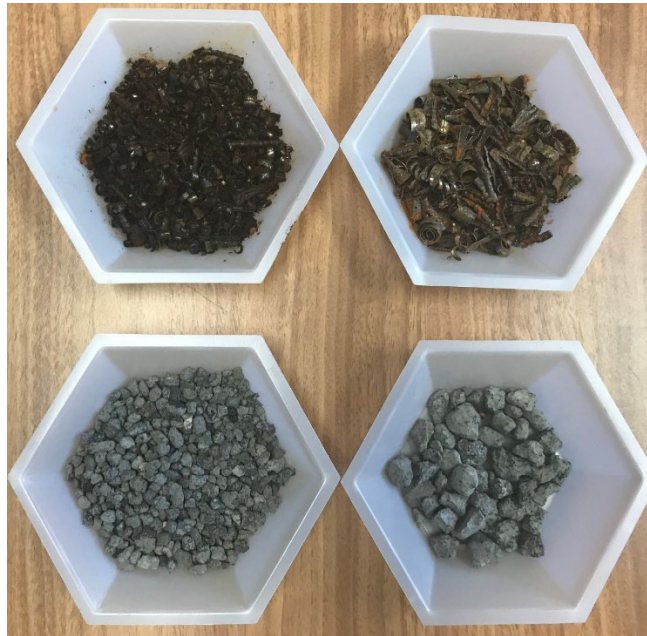
Figure 5.1 Steel chips and steel slag used for field-scale filtration study (top: steel chips 2-4 mm and 4-9.4mm, bottom: steel slag 2-4 mm and 4-9.4 mm.)
