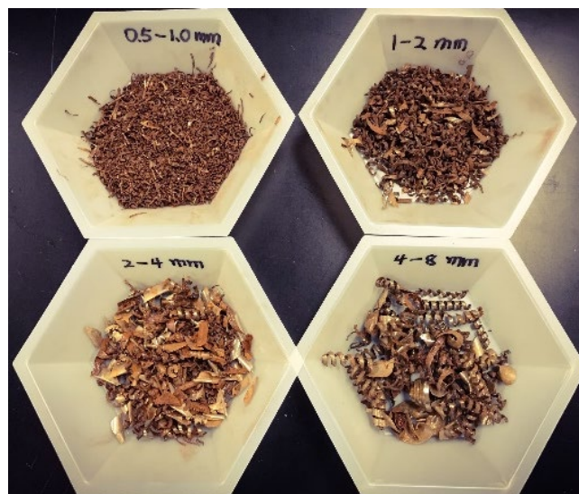
Figure 4.1 Pictures of the steel chips used for column experiments
