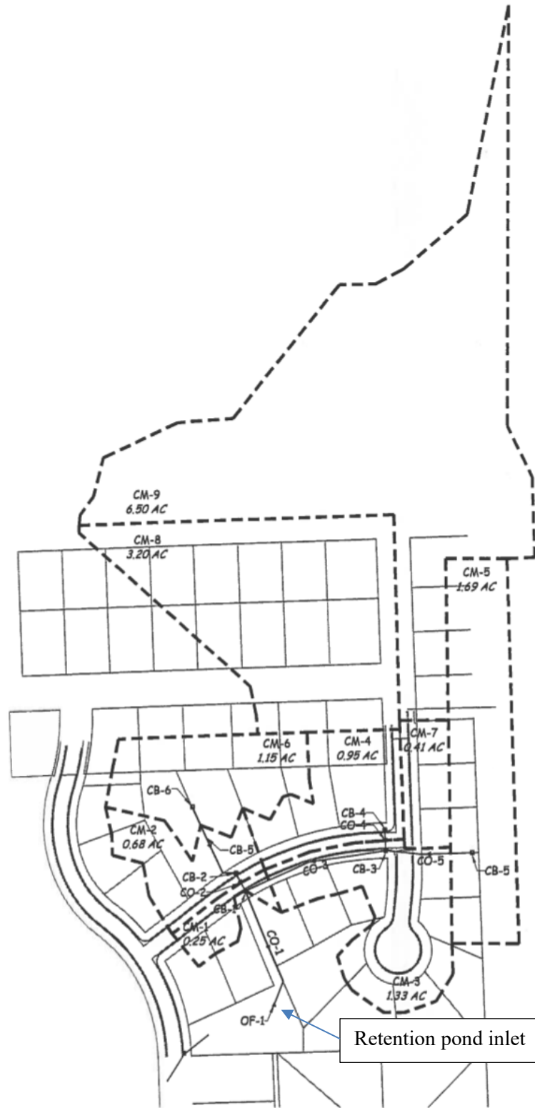
Figure 5.3 StormCAD catchments and storm sewer layout of the drainage area of the study site
