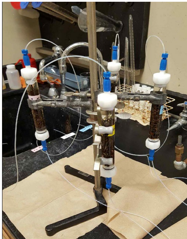
Figure 3.2 E. coli column adsorption experimental setup
