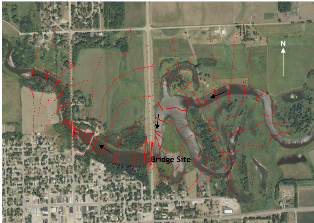
Figure 6.1 Aerial photograph of SD13 bridge site near Flandreau, South Dakota, showing the bridge crossing over the Big Sioux River and field survey points for the 2D flow model (background image courtesy of United States Geological Survey)
