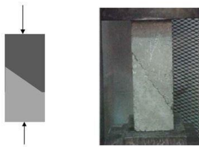
Figure 2: Slant Shear test format
