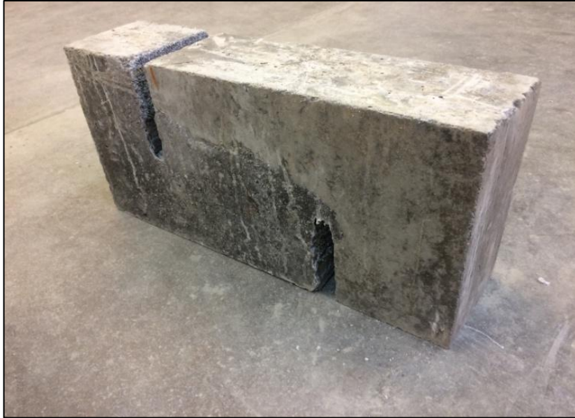
Figure 15: Composite specimen for the Double-L test after demolding
