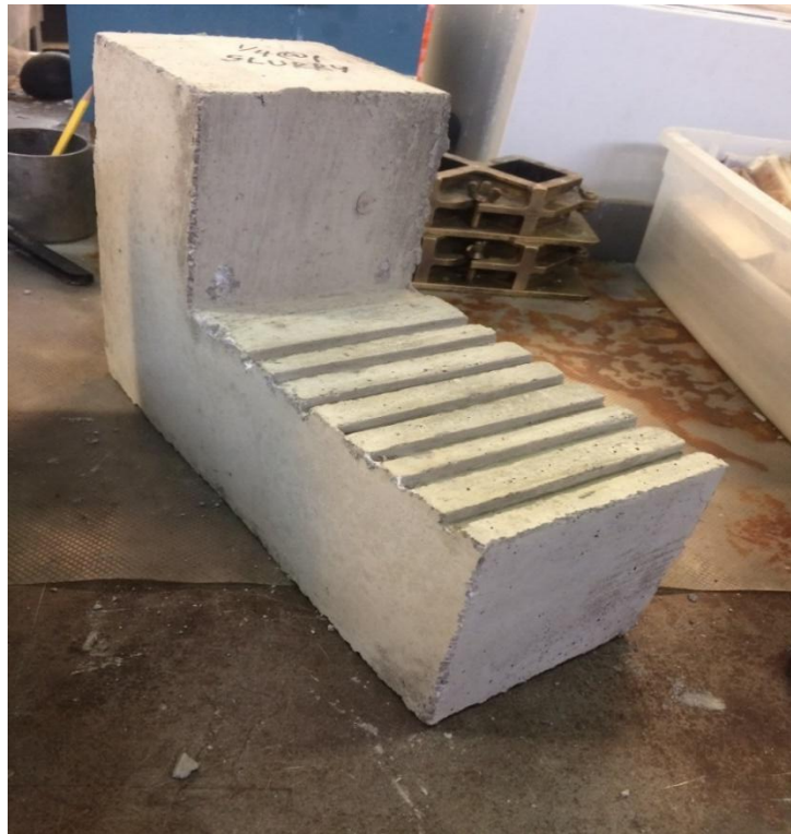
Figure 9: L-shaped underlay half after 18 hours of steam curing
