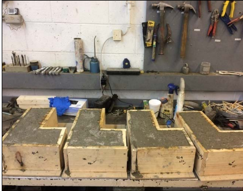
Figure 8: Freshly poured underlay concrete specimens
