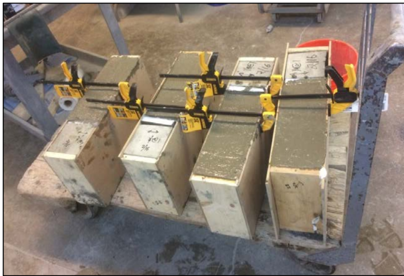
Figure 14: Composite specimen with freshly poured overlay concrete
