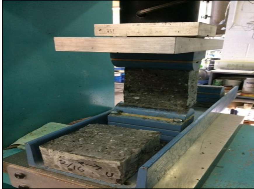
Figure 24: Composite specimen after tensile bond failure in the Split-Prism test
