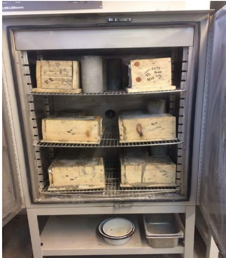
Figure 18: Underlay specimens placed in oven for steam-curing
