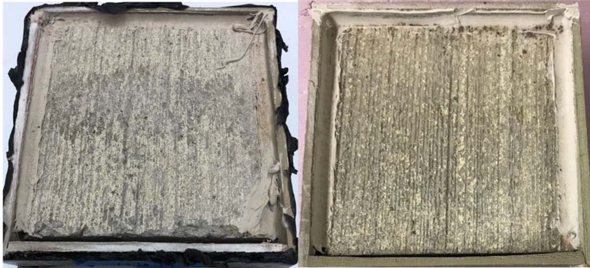
Figure 4.5.8. The Worst Performing Granite Sample After Deicer Testing G05 Untreated (left) and Silane-Treated (right)
