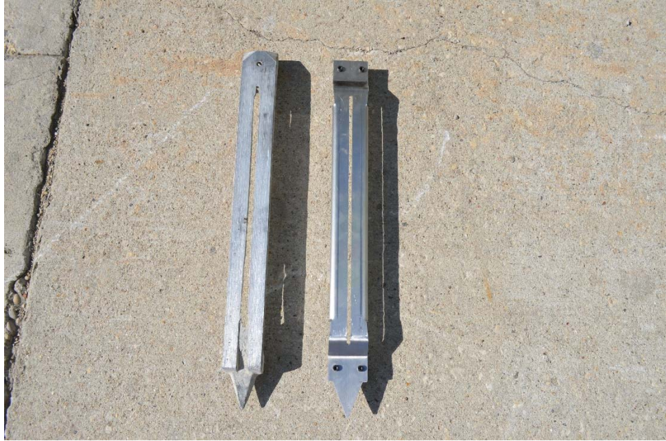
Figure 2.5.15. Old (Left) and New (Right) Plates Used During Early Entry Sawing
