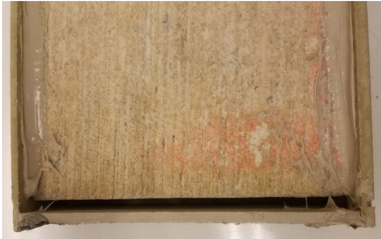
Figure 3.5.1. Deicer Scaling Sample Showing the Gap Along the Joint to Provide Deicing Solution Access
