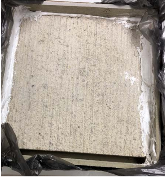
Figure 4.2.10. TTE Granite Sample of G19, Late Sawing Window for Conventional Sawing
