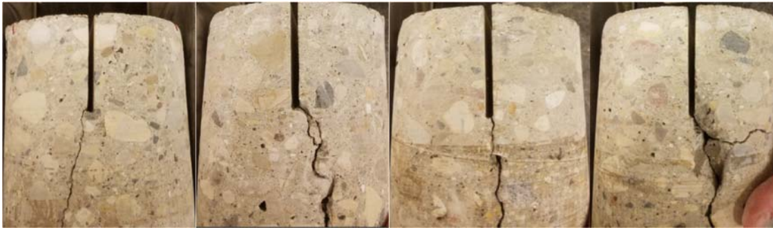
Figure 4.2.15. Core Samples Sawn to a Depth of 2.67 in. (D/3)
