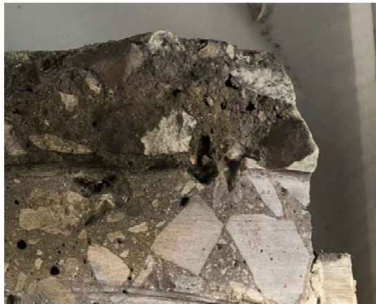
Figure 4.5.6. Chloride Penetration of Worst Performing Limestone Mixture (L16)
