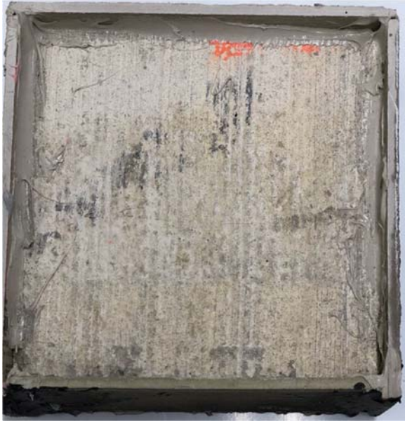
Figure 4.2.8. TTE Granite Sample of G06, Gold Standard for Early Entry Sawing
