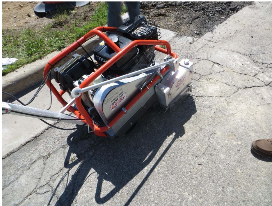
Figure 2.10.11. Husqvarna SOFF-CUT Model 2000 Early Entry Saw
