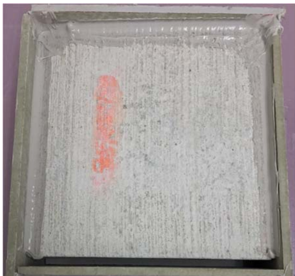
Figure 4.2.4. TTE Limestone Sample of L11, Early Window Sawing for Conventional Sawing
