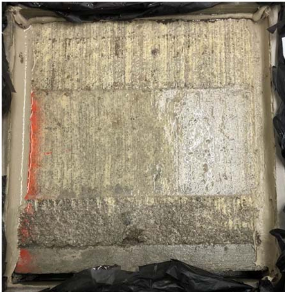
Figure 4.2.1. TTE Limestone Sample of L01, Early Window Sawing for Early Entry (surface wet)
