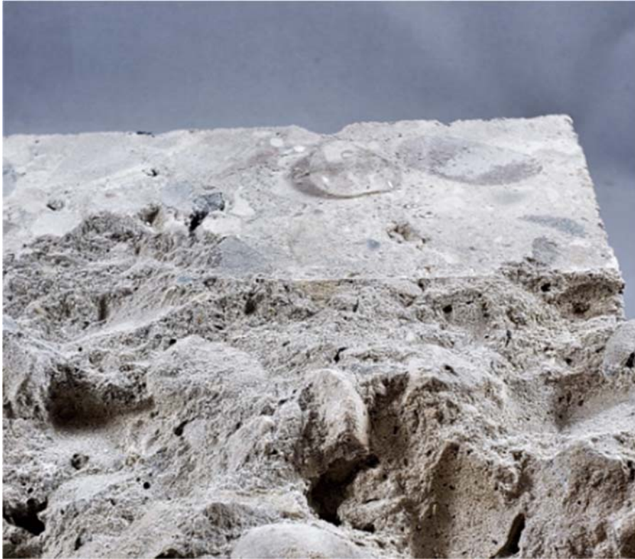
Figure 4.2.17. Sealed Core Sample Showing Hydrophobic Nature Before Testing
