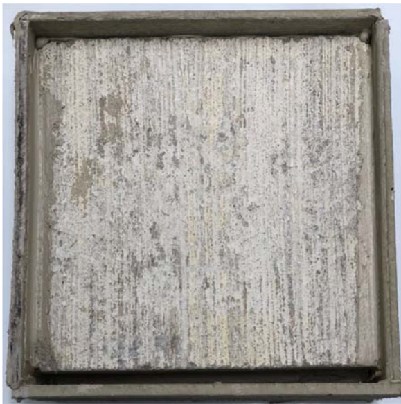
Figure 4.2.3. TTE Limestone Sample of L10, Late Window Sawing for Early Entry Sawing
