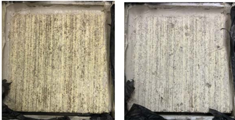
Figure 4.5.1. The Best Performing Limestone Mixture (L17) Before (left) and After (right) 50 Deicer Cycles
