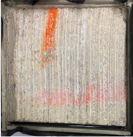
Figure 4.2.6. TTE Limestone Sample of L18, Late Window Sawing for Conventional Sawing (wet surface)
