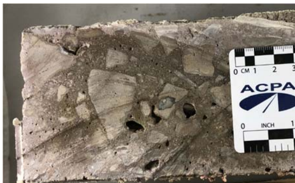
Figure 4.5.4. Chloride Penetration of the Best Performing Limestone Mixture (L17)
