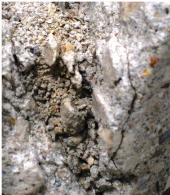
Figure 1.2.1. Slivers from Freezing and Thawing Cycle (Taylor et al., 2012a)
