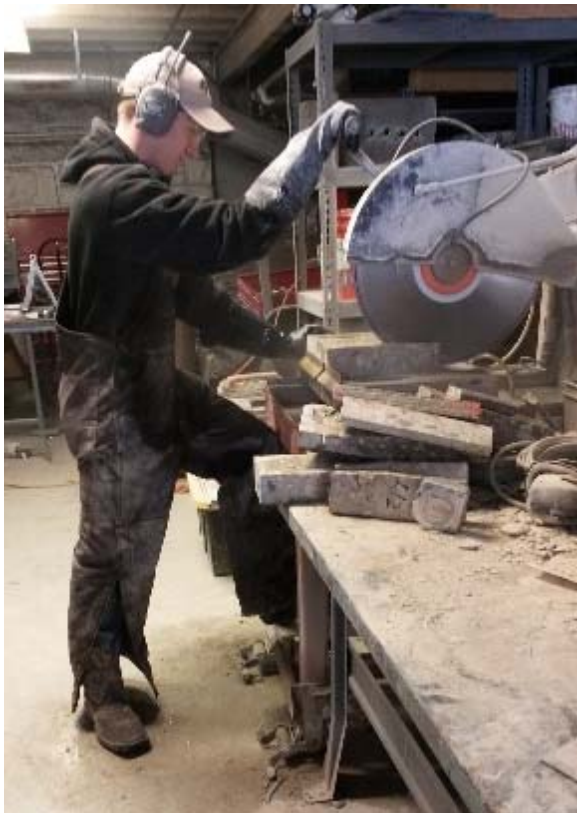
Figure 3.1.2. Final Sizing on Concrete Slab Saw
