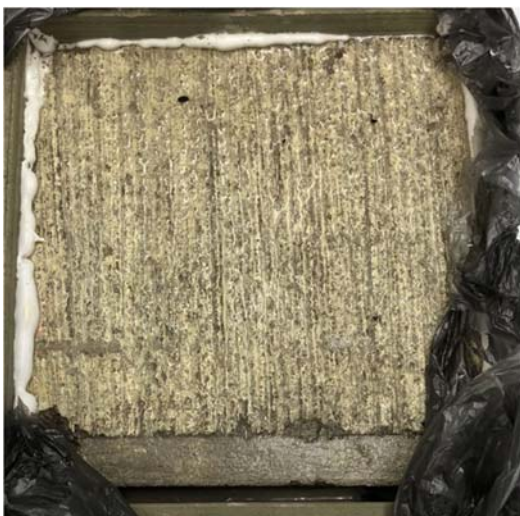
Figure 4.2.7. TTE Granite Sample of G01, Early Sawing Window for Early Entry Sawing (wet surface)
