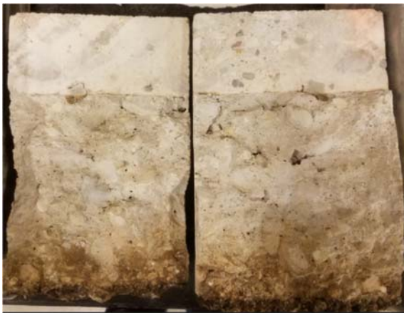
Figure 4.2.16. Core Samples Sawn to a Depth of 2.0 in. (D/4)
