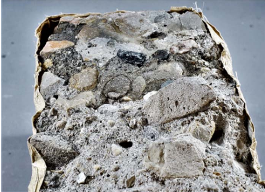
Figure 4.2.18. Sealed Core Sample Showing no Hydrophobic Nature After Freeze-Thaw Testing
