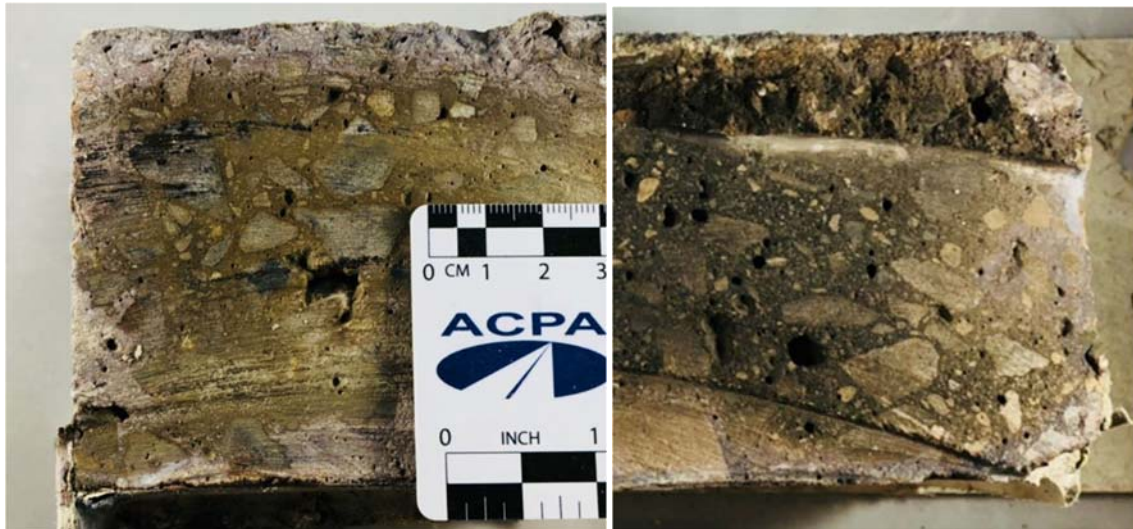
Figure 4.5.9. Chloride Penetration of G05 Untreated (left) and Silane-Treated (right)
