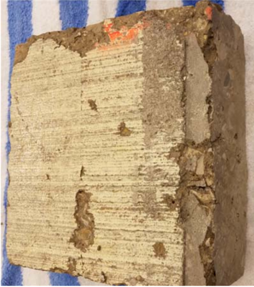
Figure 4.2.11. Joint Damage Observed for the Early Sawn Limestone Samples
