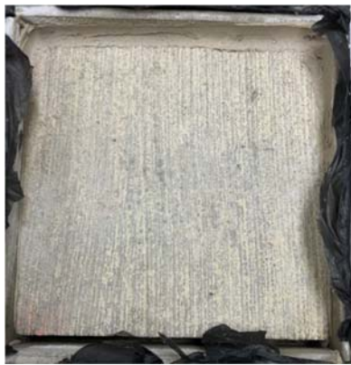
Figure 4.5.3. The Silane-Coated Duplicate Sample to the Worst Performing Limestone Mixture (L16) After 50 Deicer Cycles
