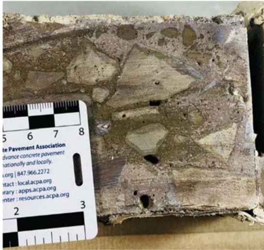
Figure 4.5.5. Chloride Penetration of Silane Coated Mixture (Ls17)
