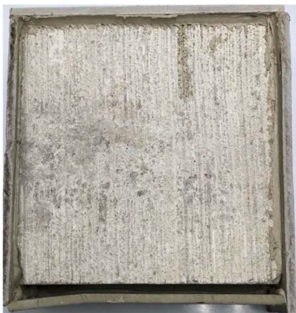
Figure 4.2.5. TTE Limestone Sample of L15, Gold Standard for Conventional Sawing
