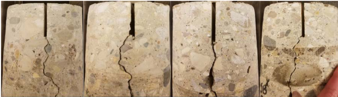
Figure 4.2.14. Core Samples Sawn to a Depth of 2.0 in. (D/4)
