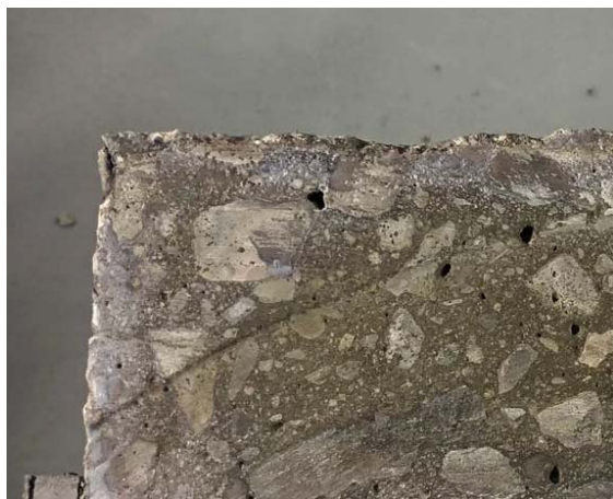
Figure 4.5.7. Chloride Penetration of Silane-Coated (Ls16)
