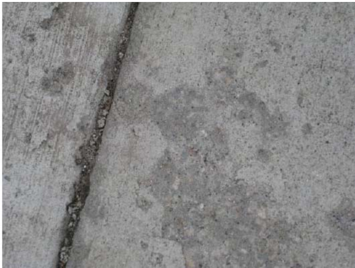
Figure 1.8.1. Salt Scaled Concrete Surface (Zhang, 2013)
