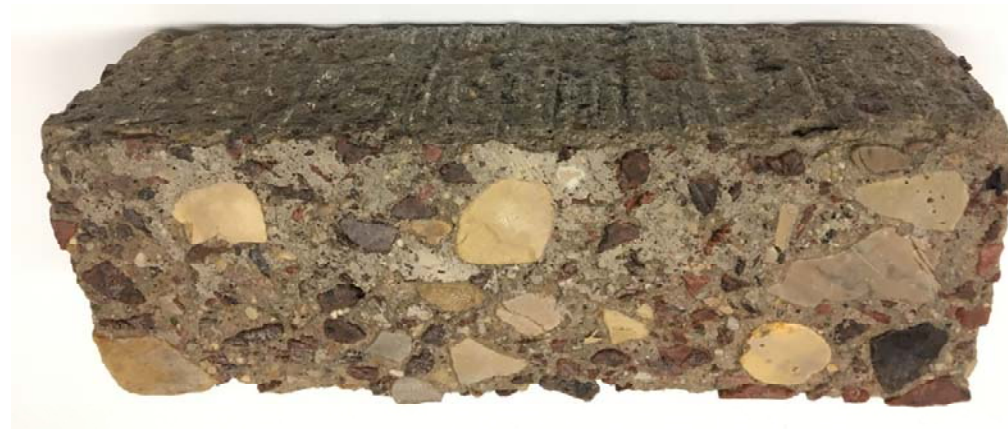
Figure 4.4.11. Granite Mixture G06 after 600 Freeze-Thaw Cycles
