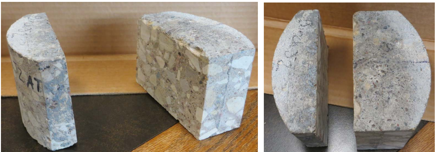
Figure 5.7.2. Typical Transverse Joint Core Specimens After Trimming (Birch J2A-J2B)
