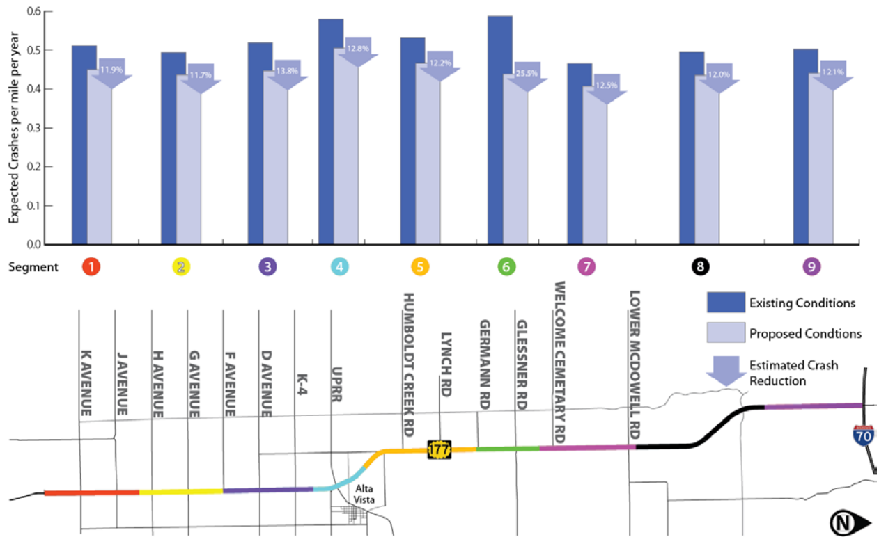
Figure 2. Projected Change in Crash Frequency on K-177 as a Result of the Modernization Project (Figure 5.5 from KDOT Project Report)
