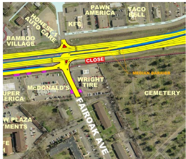
Figure 5: At-Grade RCUT Alternative with Signal Removal at Fairoak Avenue [Source: Highway 10 Access Planning Study]
