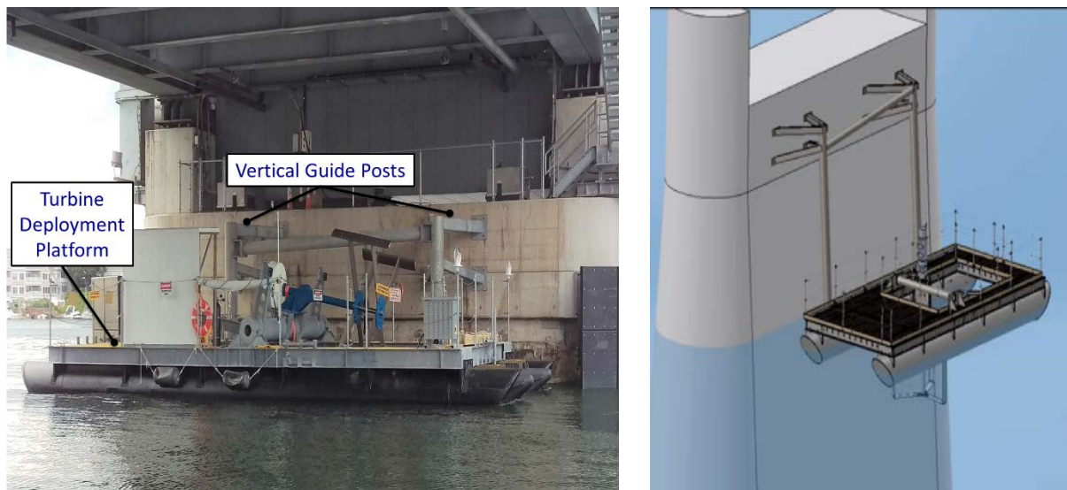
Figure 61. The tidal turbine configuration.
