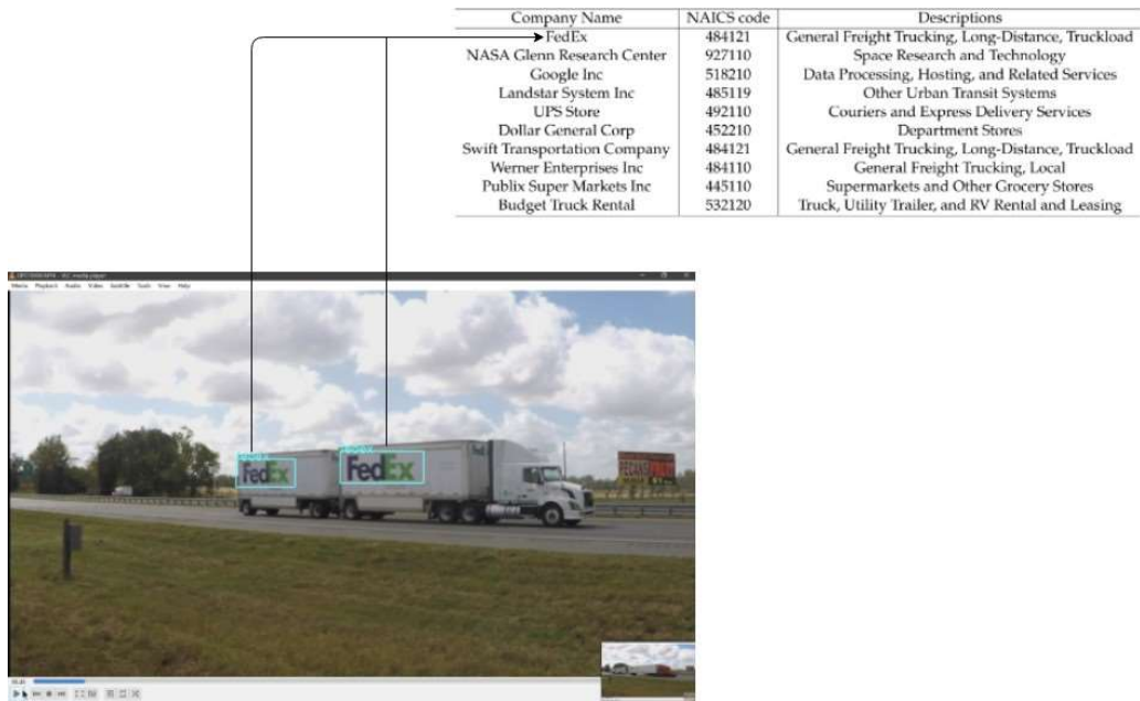
Figure 25: Example of our solution for commodity classification. Given the FedEx truck image, our developed algorithm predicted and placed the label 'FedEx' over the logo. It was then used as the query string for the U.S. company list to obtain results such as industry information (General Freight Trucking, Long-Distance, Truckload) and NAICS code 484121.
