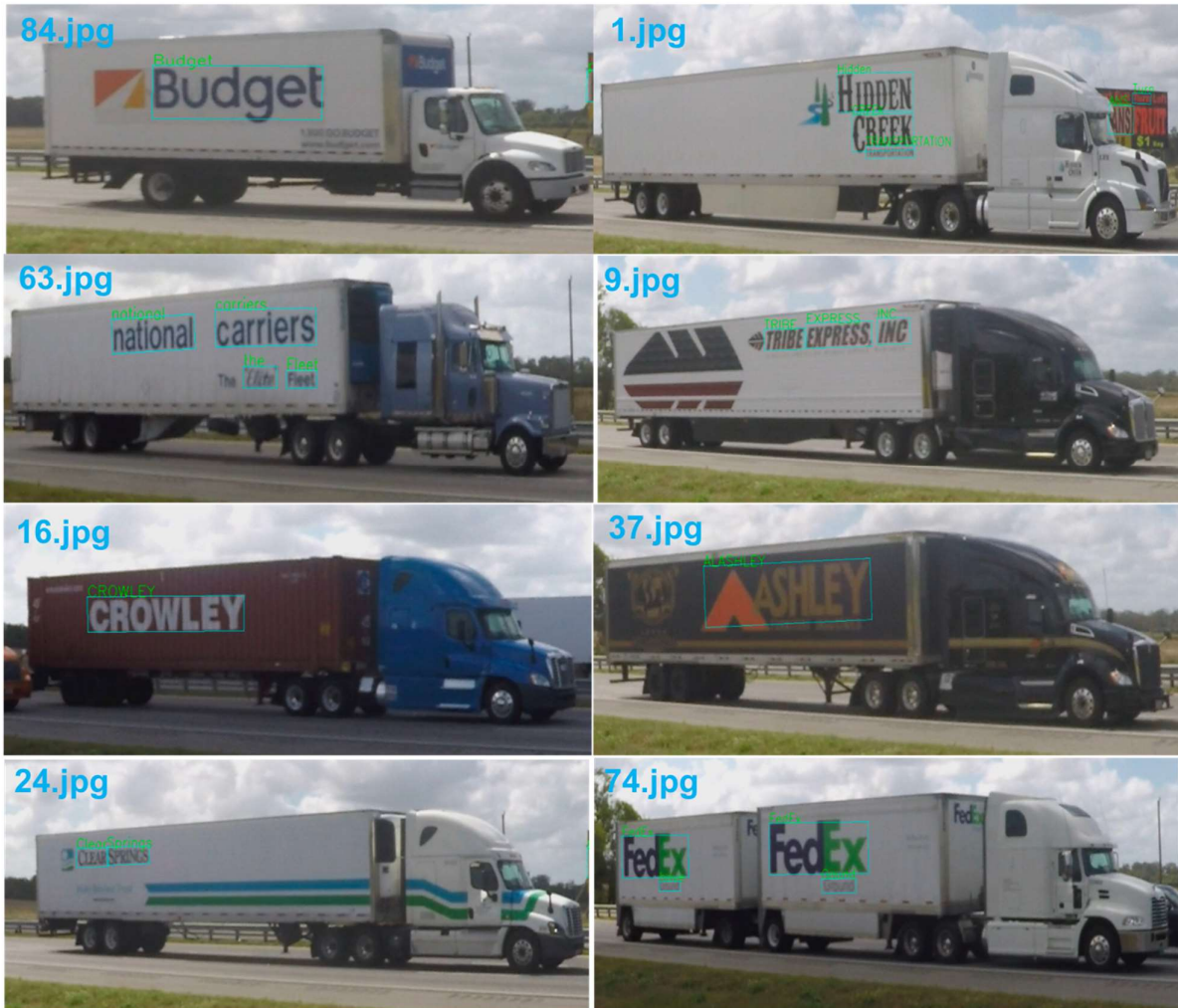
Figure 16: Results for our developed algorithms for text detection and recognition of videos from I-75 site 9956. The developed algorithms achieved a high recall with a competitive recognition accuracy. Notice that some of the recognition results missed or wrongly predicted one or a few characters, which in reality should not cause many problems because the recognition results are further processed by matching the most similar results.
