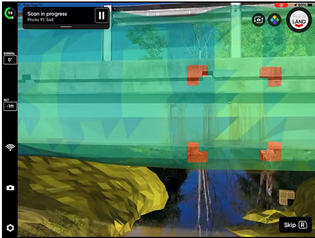
Figure 3.2.30: Skydio 3D Scan Screenshot during autonomous scan of the Beyer Road Bridge.
