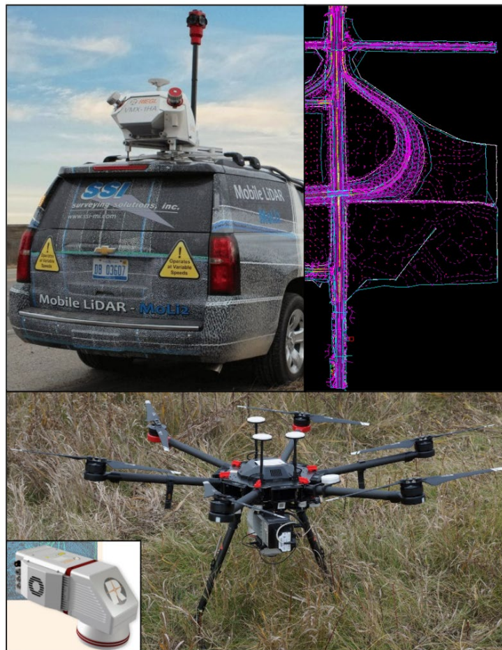
Figure 3.4.2: SSI’s MLS and UAS- based LiDAR systems (top left, bottom-right), and an example DGN file containing traditional survey data for soft surfaces.
