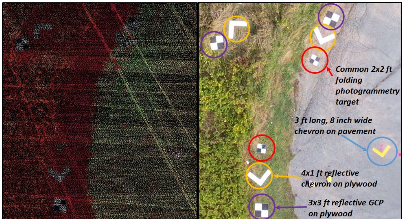
Figure 3.4.9: Lidar scan intensity cloud and drone RGB image of the same location at ‘Site A’. Reflective surfaces are much more visible in Lidar scan intensity point clouds.
