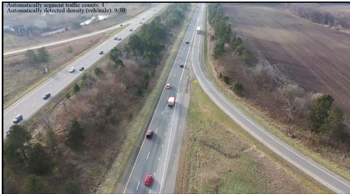
Figure 3.1.20: A screenshot of processed streaming video from Williamston Rd. on December 10, 2021. Vehicle counts and detected density are in the top left corner of the image.
