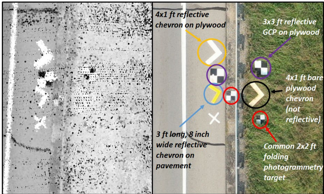
Figure 6.5.6: A selection of different ground control targets as seen in Mavic 2 RGB imagery (at right) and LiDAR point scan intensity of return data (at left) collected at US-127 over railroad site outside of Rives Junction, MI (October, 2020).
