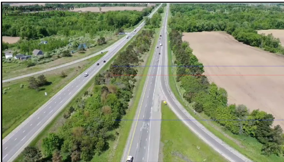
Figure 3.1.22: A screenshot of processed streaming video during this demonstration. The segment vehicle counts and cumulative vehicle counts are in the top left corner of the image.
