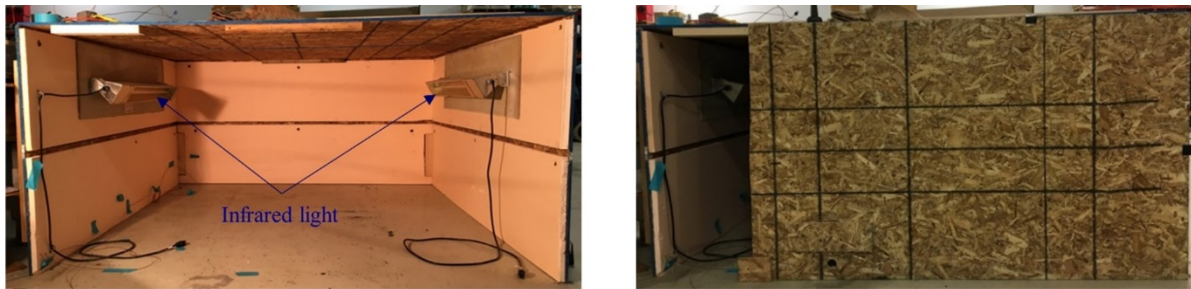
a) Insulated heating chamber with infrared lights
