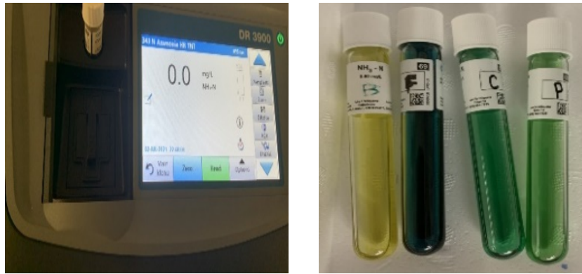
Figure 2: Ammonia Measurement Using Hack Spectrometry
