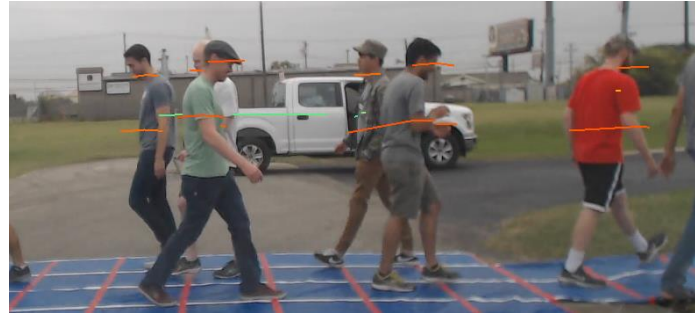
Figure 4.12: Preprocessed LIDAR measurements superimposed onto images. Top: Pedestrian’s arm is segmented as a separate measurement. Bottom: Two pedestrians are merged into a single measurement (middle pair, lower laser).
