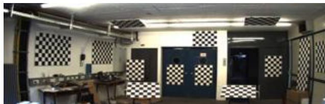
Figure 5.10: The room used to calibrate sensors to create the KITTI dataset [5.10]
