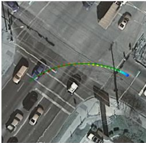
Figure 4.1: Comparison of raw GNSS measurements (dotted) to tracked vehicle positions (green line), as well as imputed speed and heading
