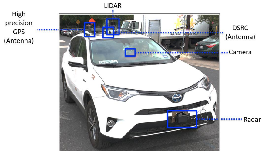
Figure A.2: Picture of car with sensors annotated
