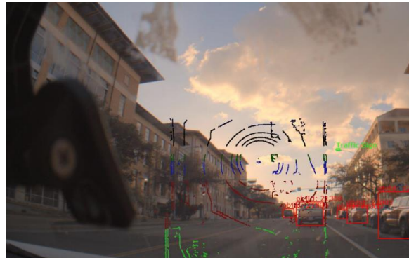
Figure 2.4: Screenshot of modified DriveWorks display, with bird's-eye view LIDAR points over the video with detected objects marked. The bottom left states the velocity of each object.
