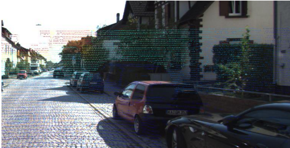
Figure 5.9: Example of bad calibration between a frontal camera and a rotational 64-layer LIDAR (KITTI dataset). Colored dots represent different distances measured by the LIDAR projected to the image’s coordinate system.
