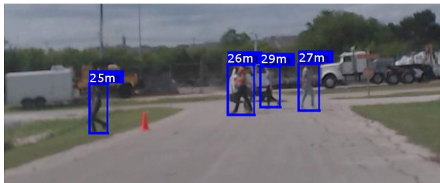
Figure 4.6: Pedestrian detection using camera in approaching vehicle
