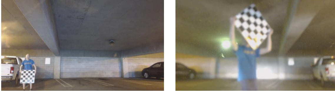
Figure 4.10: Checkerboard pictures used to determine internal camera parameters
