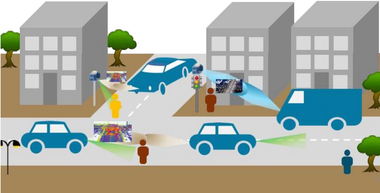
Figure 8.1: Illustration of the cellular infrastructure supporting several 5G V2X use cases enabled by mmWave communication
