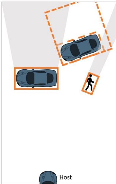
Figure 3.2: Example of partially occluded measurement, with minimum possible and maximum possible rectangles denoted with dashed lines. The gray regions are the regions that are undetectable due to the other objects.
