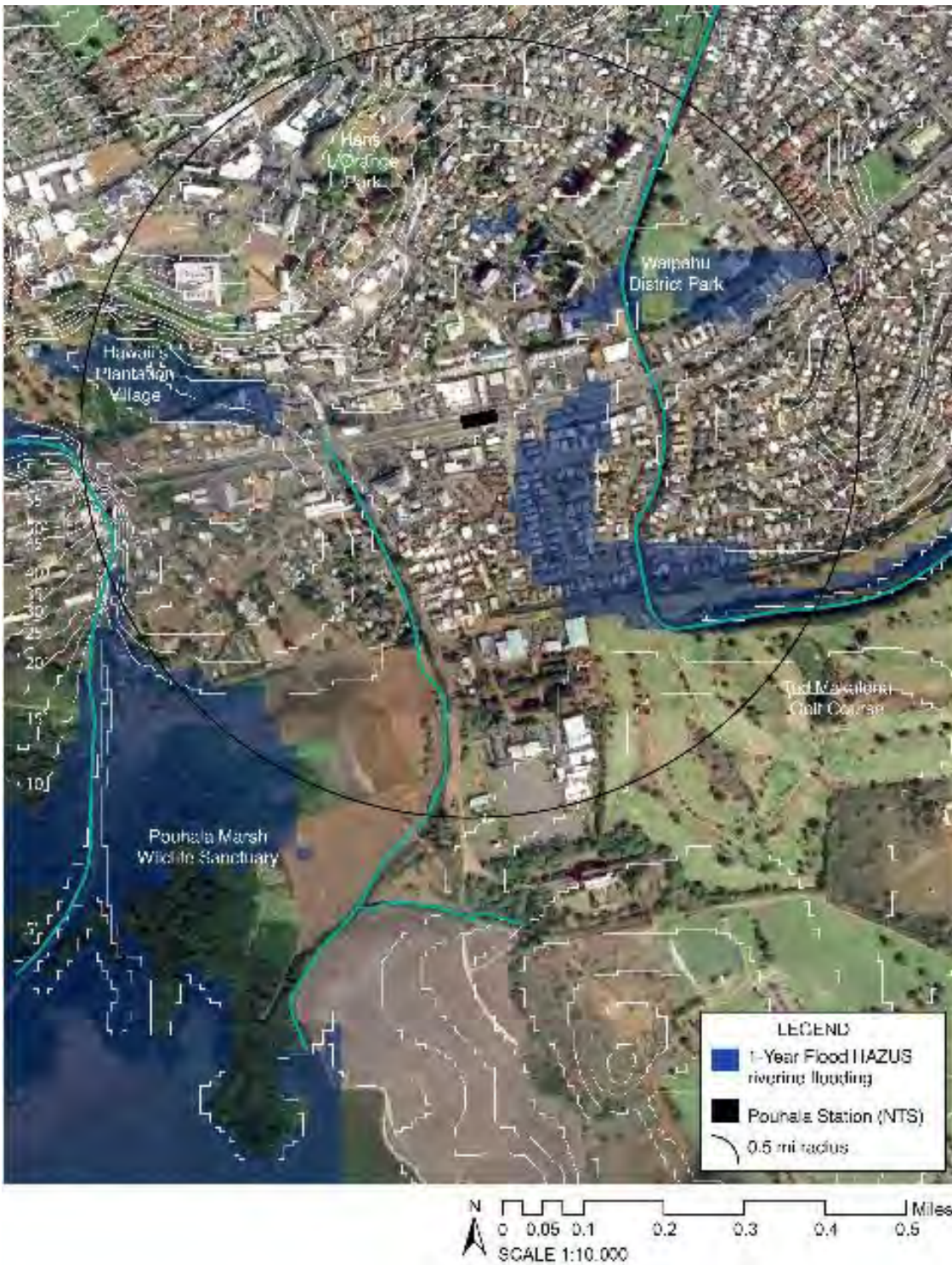
Figure 46 Waipahu TOD Site Map: Hazus Riverine Flooding Simulation – 1 Year Flood
