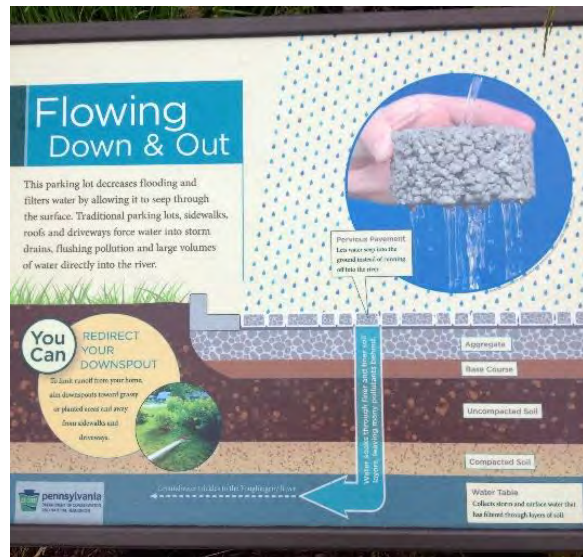
Figure 67 Illustration section drawing of permeable paving stormwater infiltration by the Pennsylvania Department of Conservation and Natural Resources. Photo: W. Meguro
