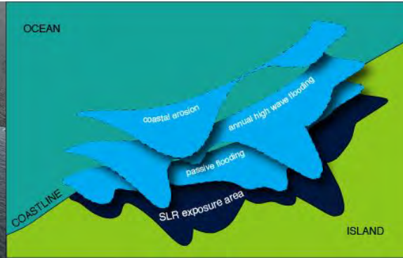
Figure 3 The SLR-XA map diagram depicts flooded areas from 3.2 ft. sea level from passive flooding, annual high wave flooding, and coastal erosion. viii
