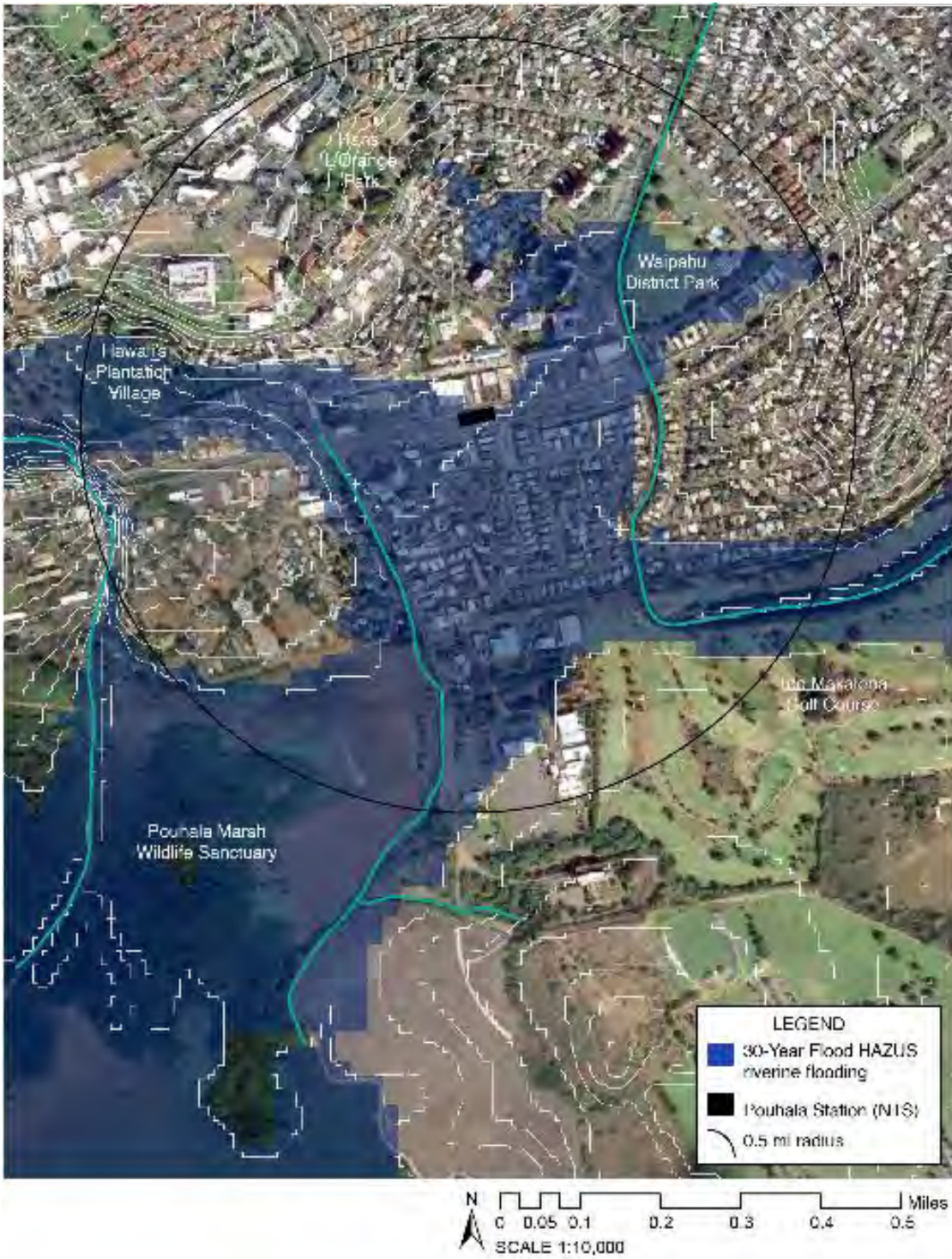
Figure 47 Waipahu TOD Site Map: Hazus Riverine Flooding Simulation – 30 Year Flood
