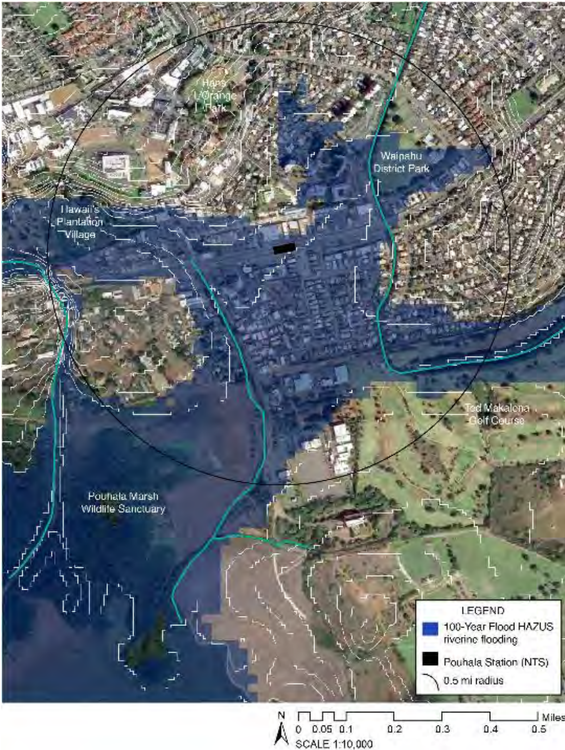
Figure 48 Waipahu TOD Site Map: Hazus Riverine Flooding Simulation 100-Year Flood
