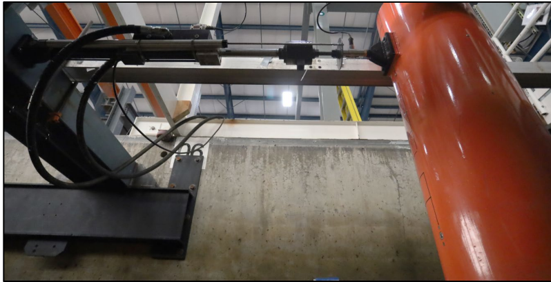
Figure 2-5. The MTS hydraulic actuator.
