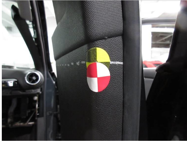
Figure D4. P9-R adjusted (red/white target) to avoid headform contact with an obstruction
