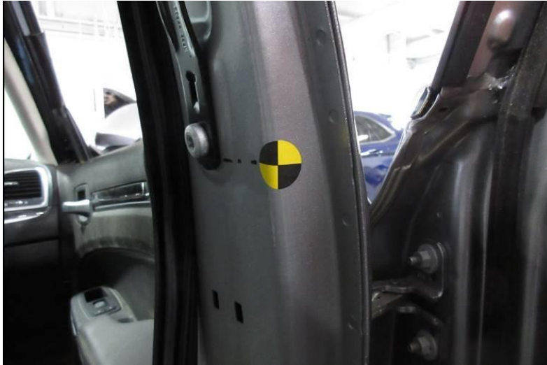
Figure D6. P9-R marked on B-pillar frame
