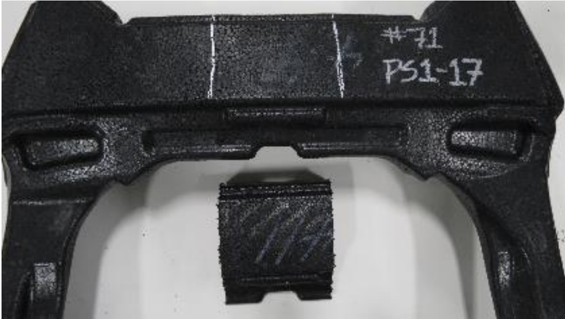
Figure 11. Jeep Grand Cherokee seat back foam bezel
