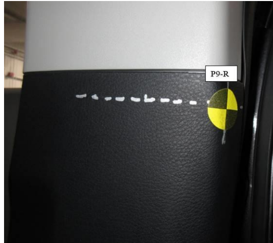
Figure D3. P9-R impact location on B-pillar trim
