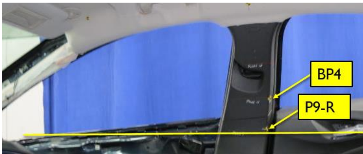
Figure 29. Lower B-pillar impact locations
