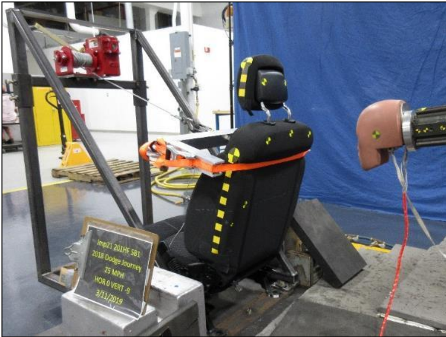
Figure 16. Setup of impacts with forward force exerted on seat backs
