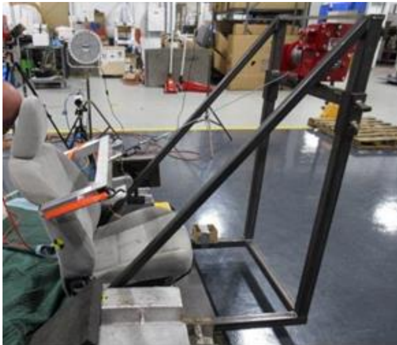
Figure C4. Seat load fixture
