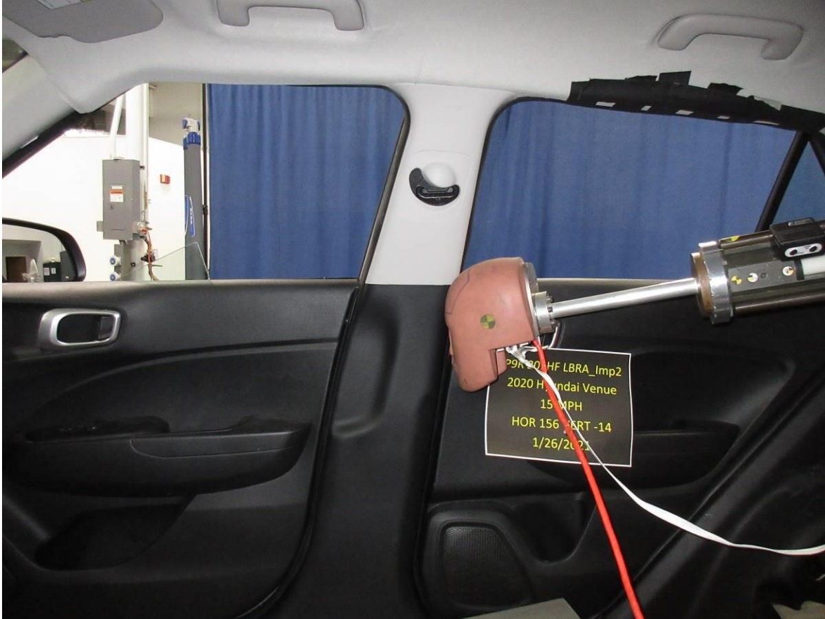
Figure D7. Position impactor to match the vertical and horizontal angles for impact
