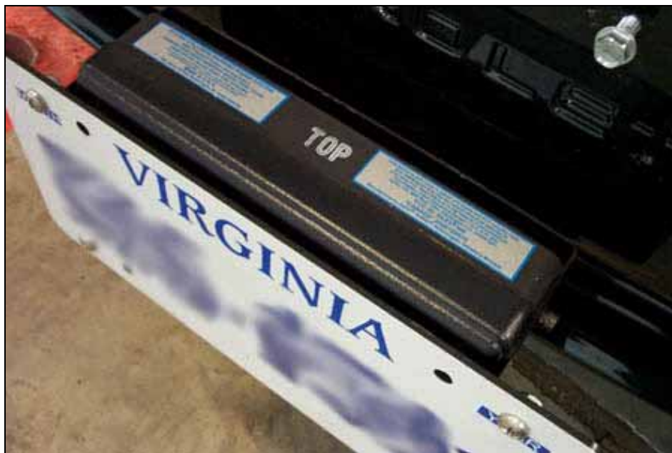
Figure 1.3. Doppler radar antenna mounted on the front of a vehicle, covered by a mock-up of one of the plastic license plates used for the study.
