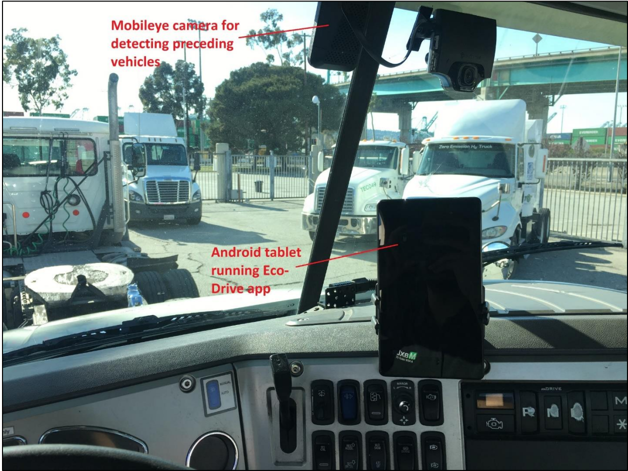
Figure 27. On-board hardware of UCR’s truck EAD system
