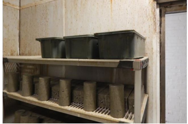
Thawing of laboratory samples (moist room)
