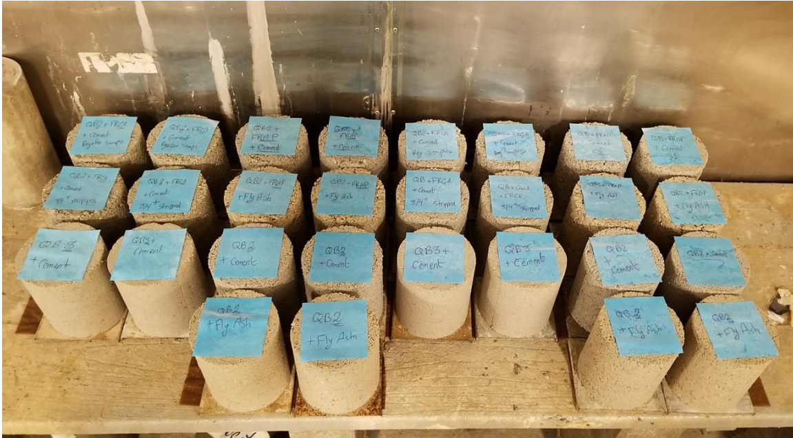
Figure 3.5. Moist room curing of the laboratory-molded samples for freeze-thaw and wet-dry durability testing.
