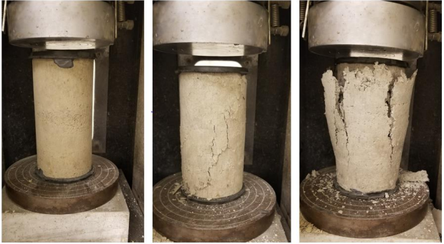
Testing of UCS samples
