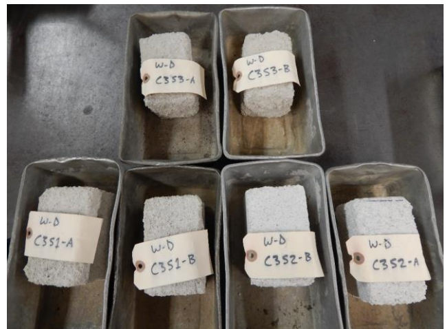
Testing of field-extracted samples for wet-dry durability
