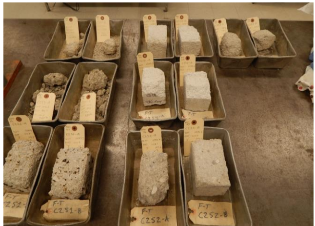
Testing of field-extracted samples for freeze-thaw durability
