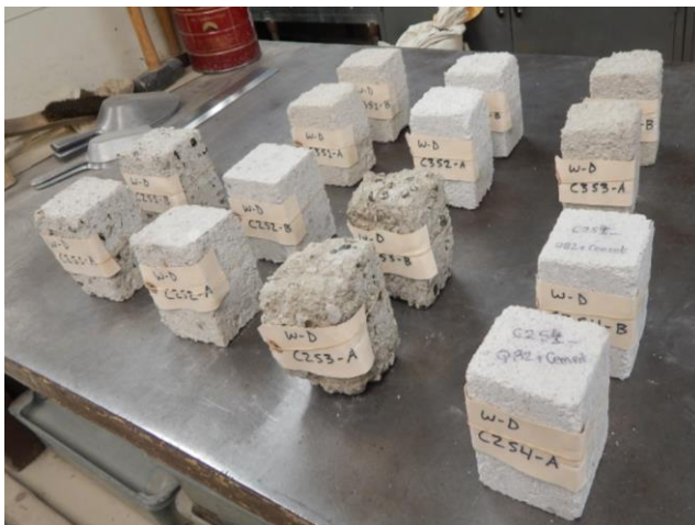
Testing of field-extracted samples for wet-dry durability
