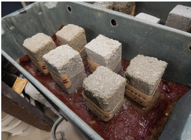
Testing of field-extracted samples for freeze-thaw durability
