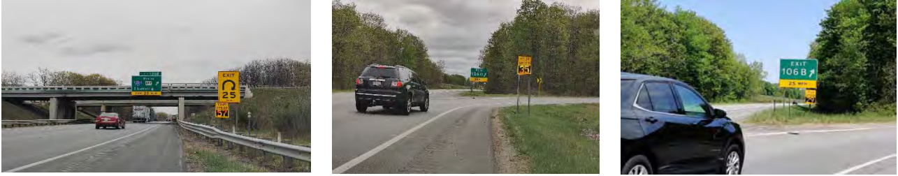
a. DSFS at advisory speed sign b. DSFS at PC (side-mount) c. DSFS at PC (fwd-mount)
