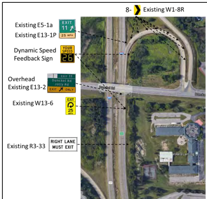
Figure 24. NB US-127 exit ramp to Dunckel Rd (Site 5)
