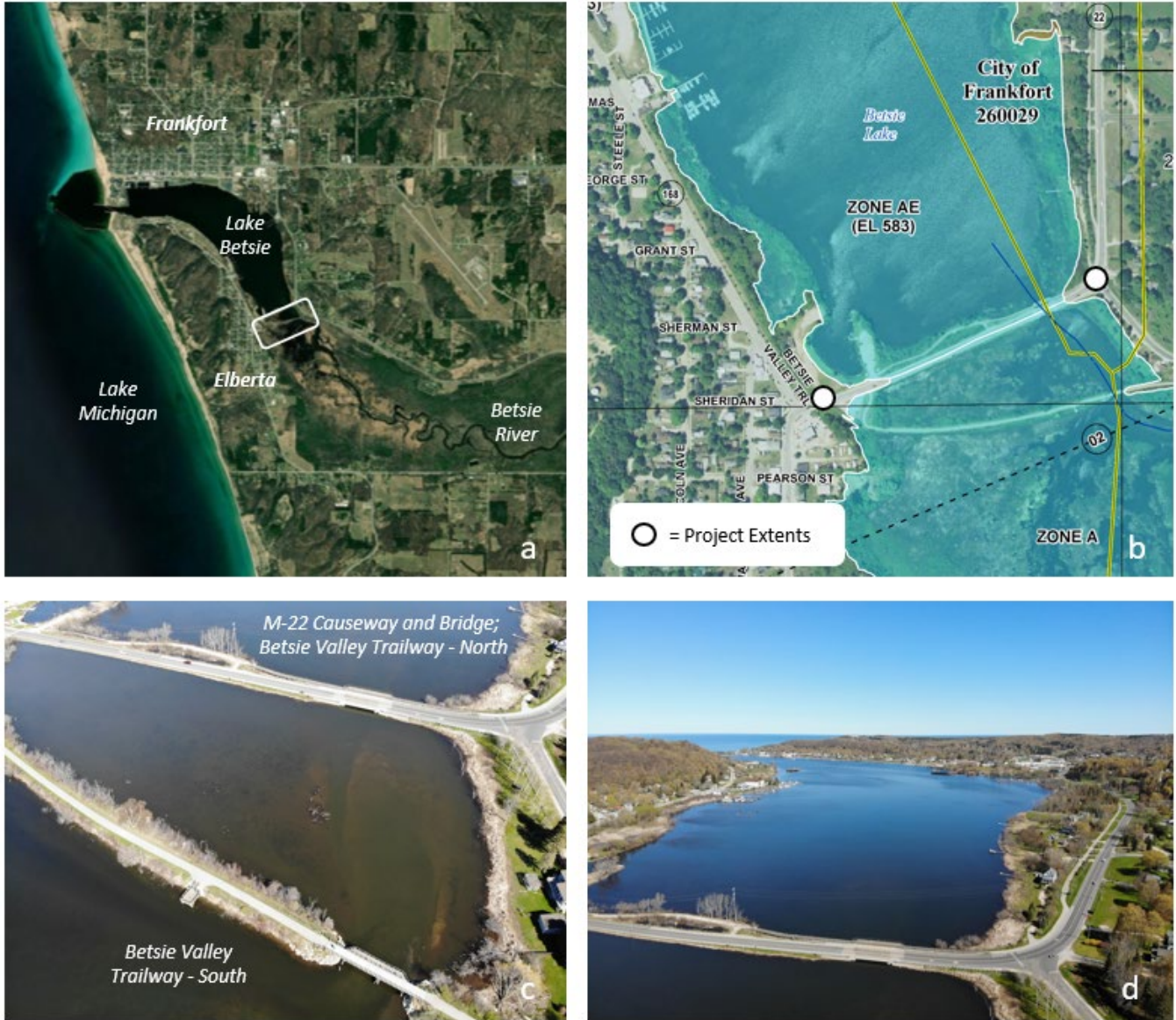
Figure 4-1. Overview of M-22 Elberta/Frankfort site and surrounding context. a) Region aerial photograph depicting relation of Betsie River, Betsie Lake, and Lake Michigan (not to scale). b) FEMA flood map showing AE and A flood zones in relation to project extents, c) the larger Betsie Valley Trailway bridge opening to the south of the site, d) aerial overview of site and surrounding context, looking toward Lake Michigan.
