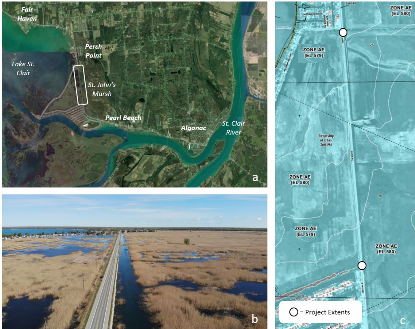
Figure 4-6. Overview of M-29 St. John's Marsh site and surrounding context. a) Region aerial photograph depicting relation of St. Clair River, Lake St. Clair, and St. John's Marsh (not to scale). b) FEMA flood map showing 580 NAVD88 and 579 NAVD88 AE flood zones in relation to project extents, c) aerial overview of site and surrounding context, looking north toward Perch Point.
