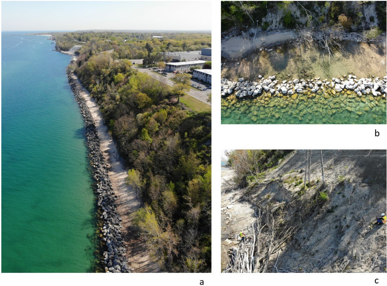
Figure 4-13. Drone imagery of I-94 BL St. Joseph, May 2021, showing a) the roadway in relation to the bluff and existing mitigation measures, b) existing state of rip-rap mitigation measures, and c) evidence of slope failure.
