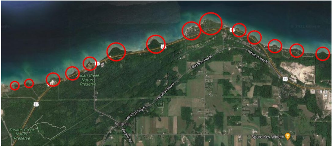
Figure 4-18. V-shaped land protrusions into Little Traverse Bay west of Bay Shore, Michigan, that may be evidence of previous slope/bluff failures on the southern shore of Little Traverse Bay (image modified from Google).
