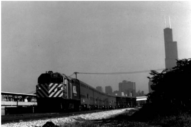
This locomotive-hauled METRA commuter rail train in Chicago uses double-deck cars, as do all commuter rail agencies in western and southern states. Clearances on old tunnels and bridges in northeastern states, however, generally allow only single-deck cars.
