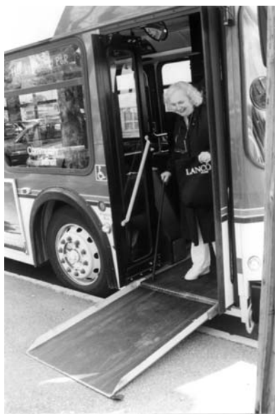
Community Transit in Snohomish County, Washington operates low-floor buses with a floor only 12-16 inches off the ground that use an extendable ramp for wheelchair access.
