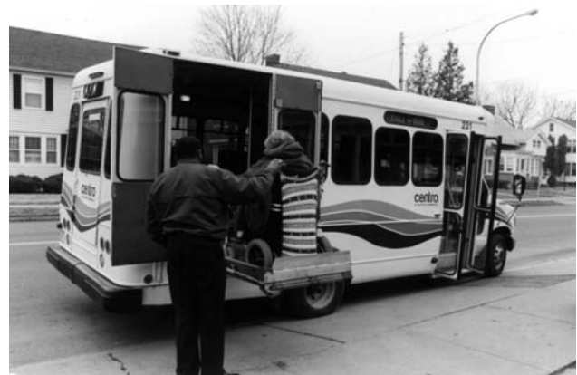
The Syracuse, New York CNY Centro system uses this typical demand response vehicle to transport persons with disabilities who are unable to use its fixed route buses.
