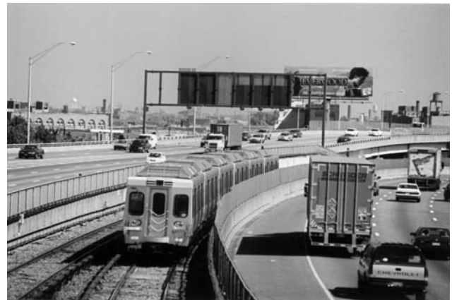
A Philadelphia Southeastern Pennsylvania Transportation Authority train operates in a freeway median. When counting vehicle miles and hours for trains, each car is counted, so this 6-car train operates 6 vehicle miles for each mile traveled and 6 vehicle hours for each hour in service.
