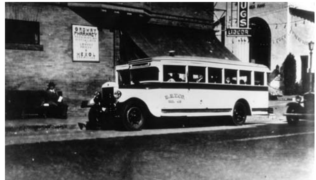
This Monterey, California bus still used in 1939 typified early buses. It wasn't until the 1930s that the engine-in-rear, flat-front design seen today became common.
