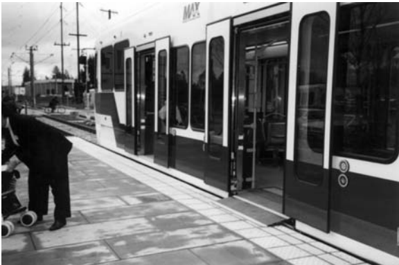
Portland's Tri-County Metropolitan Transportation District of Oregon is one of several light rail agencies to operate low-floor light rail cars.
