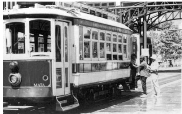
This Memphis Area Transit Authority historic light rail car in Tennessee is a high-floor car with steps at both ends.
