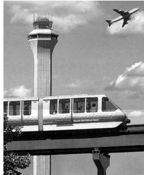
The Newark Airport AirTrain in New Jersey uses monorail technology, but is an automated guideway since the trains do not have operators.
