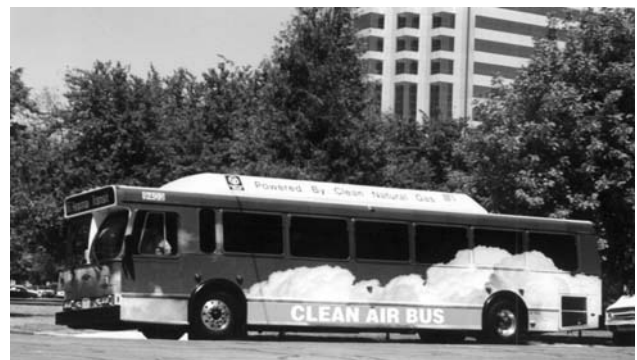
This compressed natural gas bus is operated by the Sacramento Regional Transit District in California.
