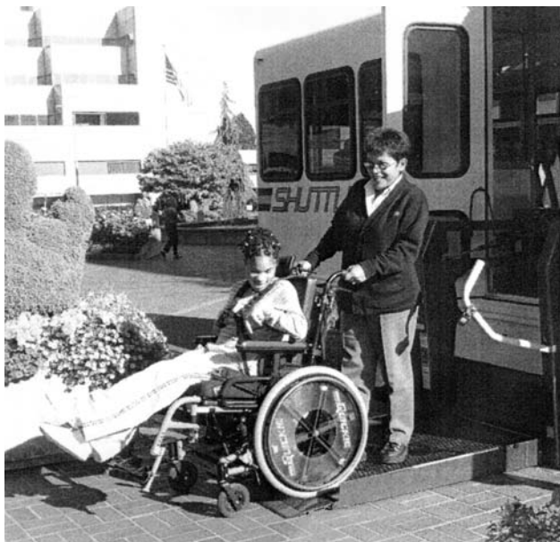
Wheelchair lift operating on a Pierce Transit van in Tacoma, Washington.
