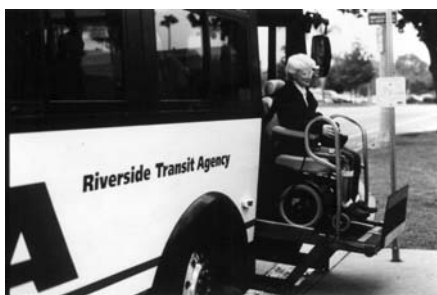
Traditional high-floor buses with steps such as this one at Riverside Transit Agency in California use lifts to accommodate wheelchair users.
