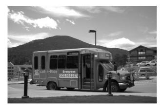
A typical body-on-chassis van operated by the Regional Transportation District in Denver, Colorado. Although this particular van is being used for demand response service, this type of vehicle is often used for lightly-patronized fixed route service.
