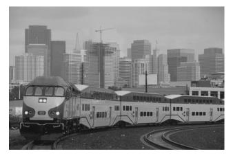
This locomotive-hauled Caltrain commuter rail train which operates in the San Francisco area uses double-deck cars, as do all commuter rail agencies in western and southern states. Clearances on old tunnels and bridges in northeastern states, however, generally allow only single-deck cars.
