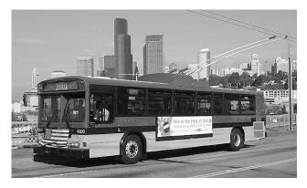
This trolleybus is a rubber-tired vehicle without an engine that is powered from two electric wires. Only five cities have them; this one is operated by the King County Department of Transportation in Seattle, Washington.
