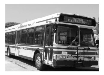
This Torrance Transit System hybrid-electric bus in California operates by combining fossil fuel and electric power technologies.
