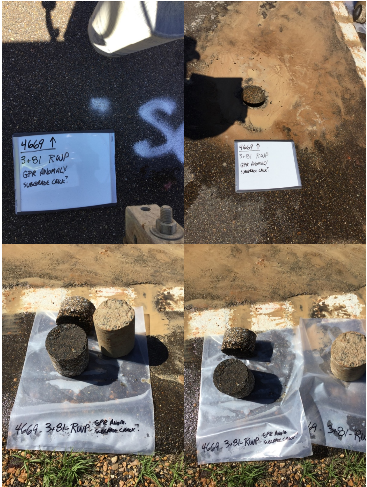
Figure 6: Core Cut at Station 3+81 – Section 4669
