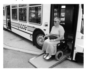
This Pace bus, which services the suburbs of Chicago, Illinois, has a low floor and is equipped with a ramp.
