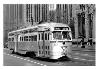
This San Francisco Municipal Railway light rail vehicle is powered by overhead electrical wires.
