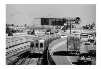
A Southeastern Pennsylvania Transportation Authority train in Philadelphia, Pennsylvania, operates in a freeway median. When counting vehicle miles and hours for trains, each car is counted, so this 6-car train operates 6 vehicle miles for each mile traveled and 6 vehicle hours for each hour in service.
