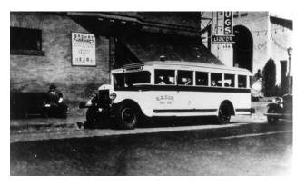
This Monterey, California bus still used in1939 typified early buses. It wasn't until the 1930s that the engine-in-rear, flat-front design seen today became common.
