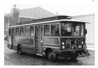
Often called a trolley, this vehicle that imitates an old streetcar is called a "trolley replica bus." Its data are included with bus statistics since it is rubber-tired and has an on-board power source. This is a Sioux Falls Transit vehicle in City of Sioux Falls, South Dakota.
