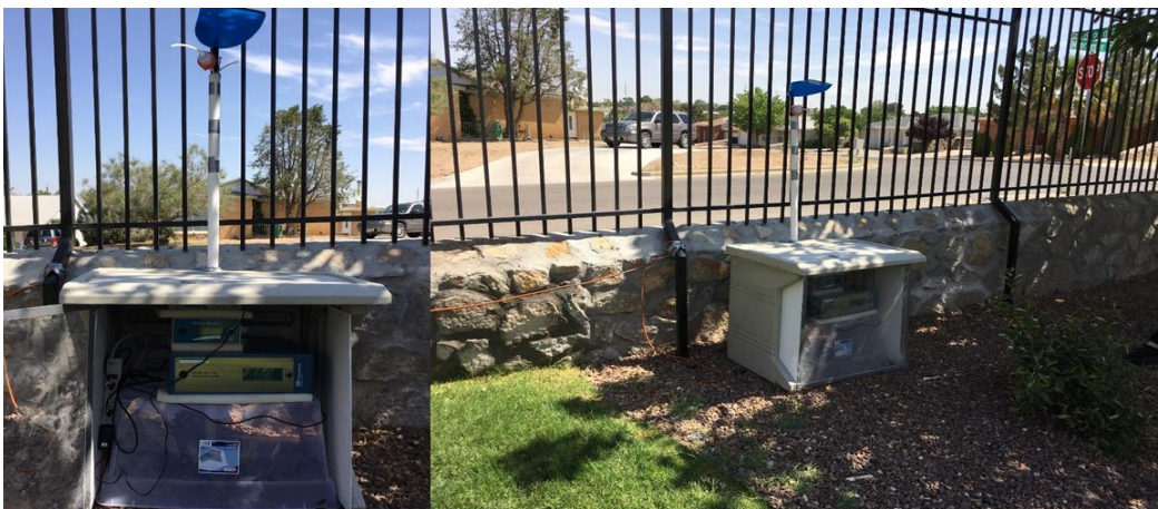
Figure 7 Air Quality Monitor Set-Up: Radford School
