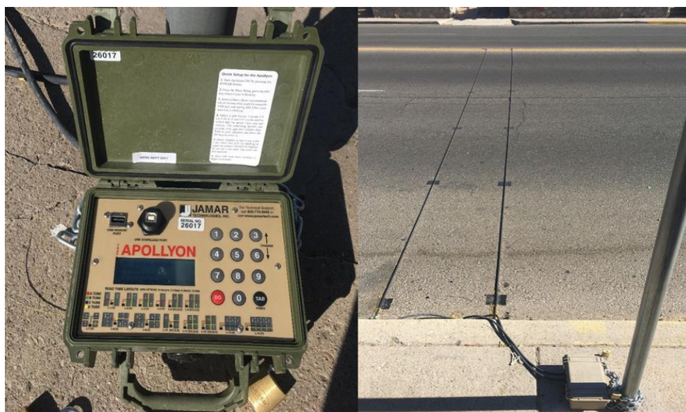
Figure 3 Tube Counters On-Site (Pershing Location)
