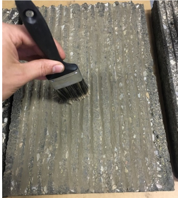
Figure 4.5: Dust being applied to pavement surface.
