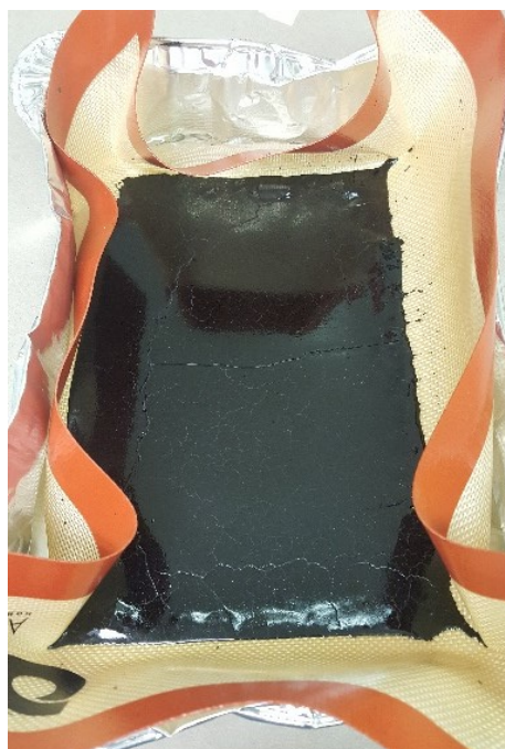
Figure 3.4. Tack coat binder after low temperature distillation
