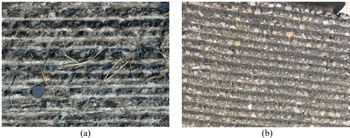
Figure 3.2: Comparison of milled pavement surfaces (a) in the field (Mokarem 2006) and (b) in the laboratory.
