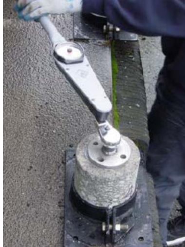
Figure 2.25: Torque bond test device (Tashman et al. 2006).
