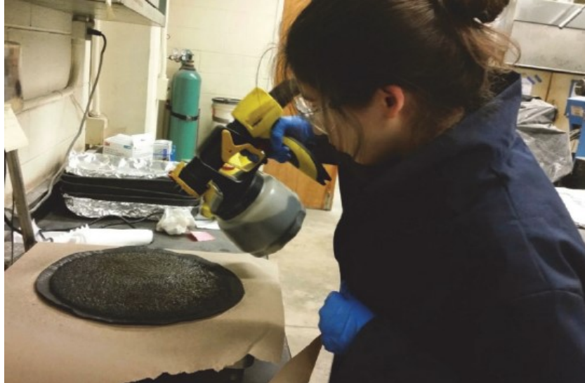
Figure 2.13: Application of tack coat in the laboratory (Rawls et al. 2016).
