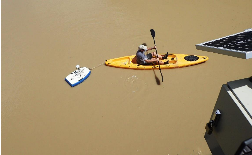
Figure 3-8 The M9 ADCP attached to a kayak to collect flow and bathymetry
