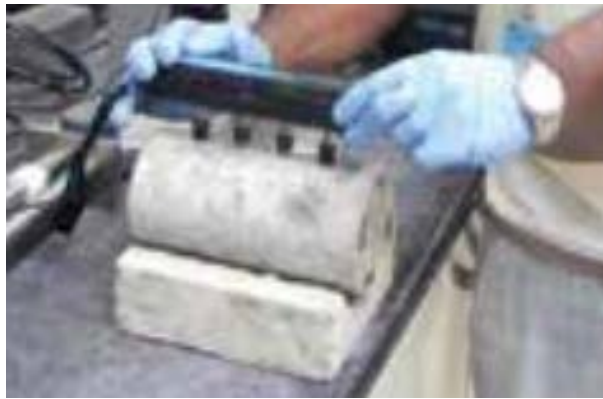
Figure 2. Measuring permeability using surface resistivity method.
