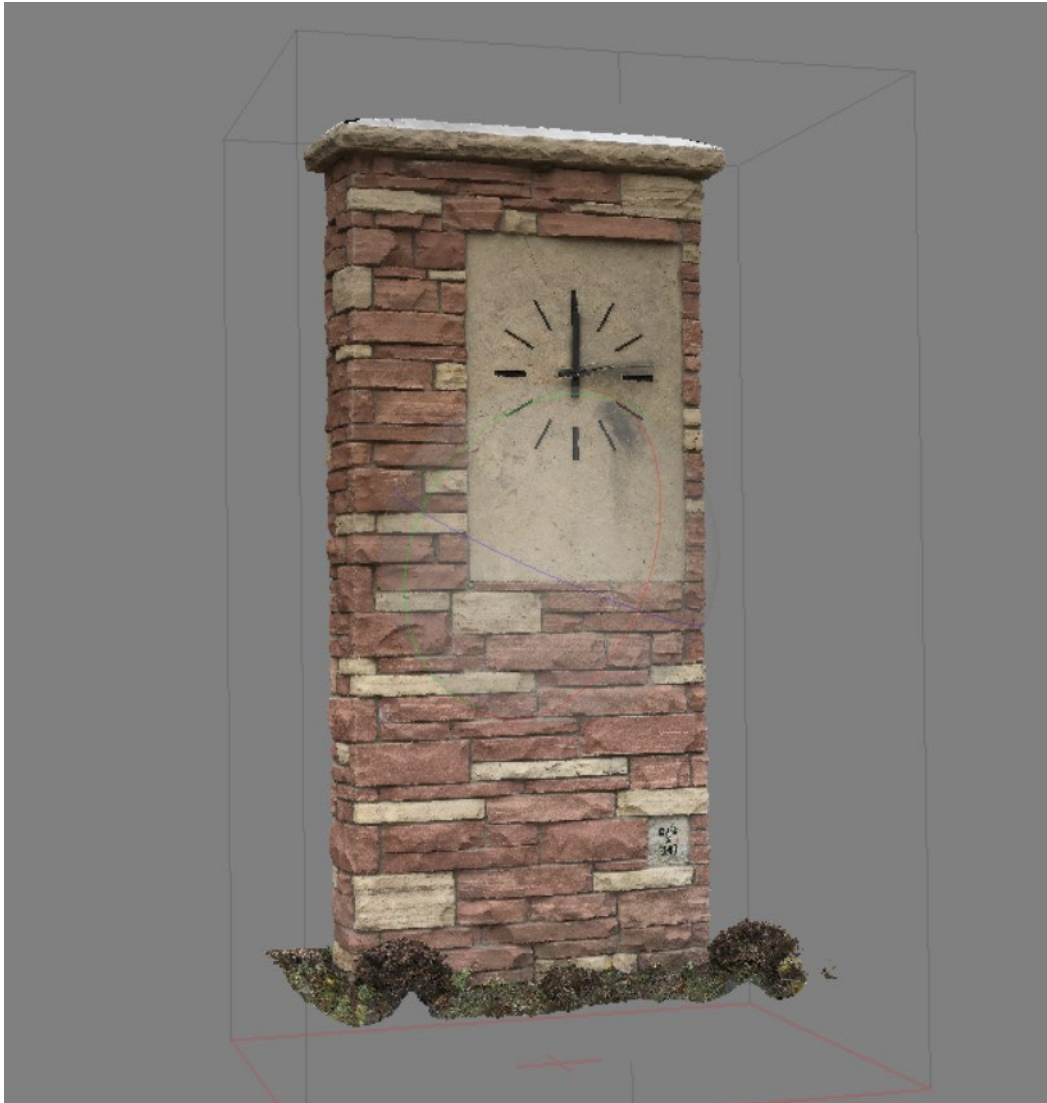
Figure 2.2 The point cloud of clock tower generated by Photoscan
