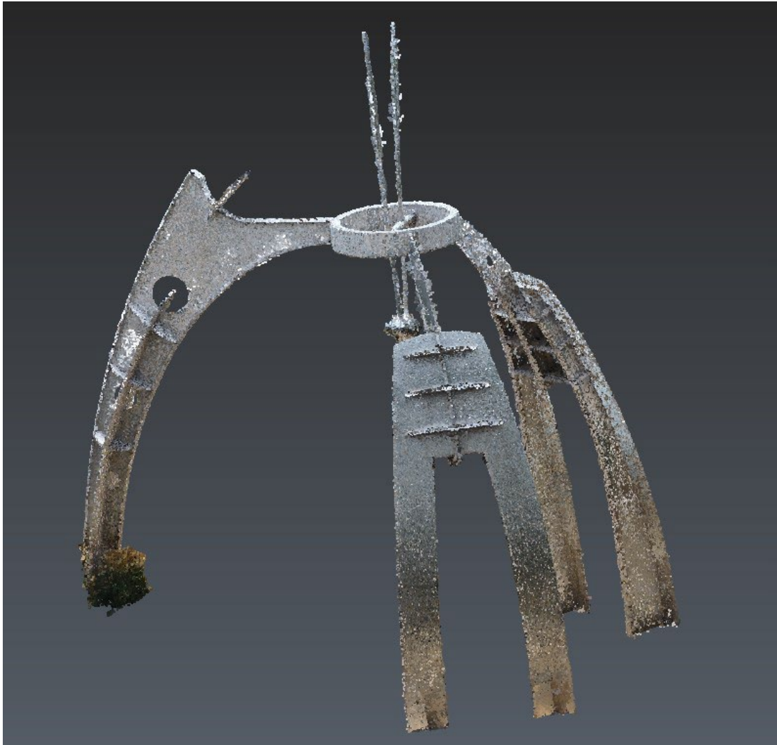
Figure 2.7 The refined point cloud by using 3DReshaper
