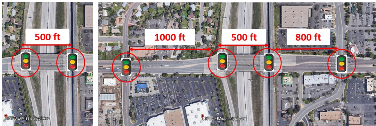
Figure 1.2 Network-1 showing two intersections (left image) and Network-2 showing four intersections (right image)
