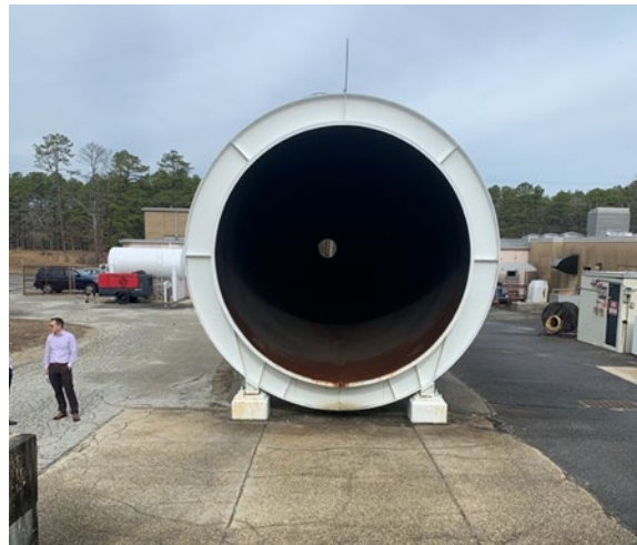
Figure 11. Exhaust port behind FAA wind tunnel for disturbance flight testing
