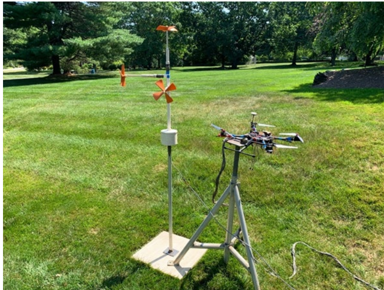
Figure 7. Instrumented Tarot 650 on sting balance with 3-axis anemometry stand
