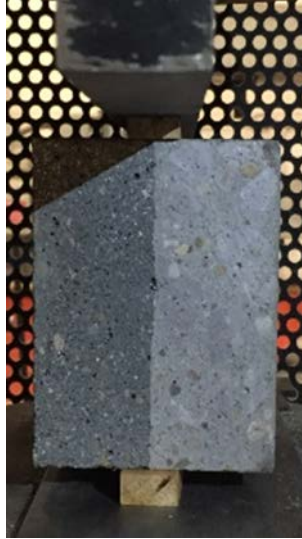
Figure 6. Split prism test setup.
