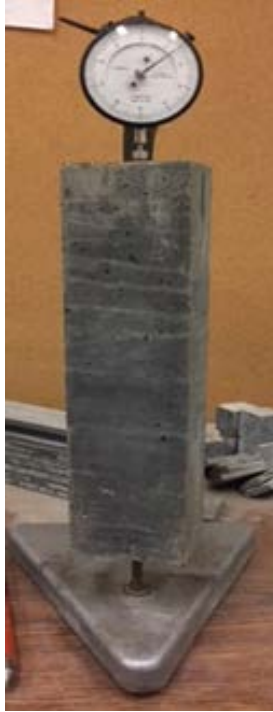
Figure 10. Longer-term shrinkage test setup.
