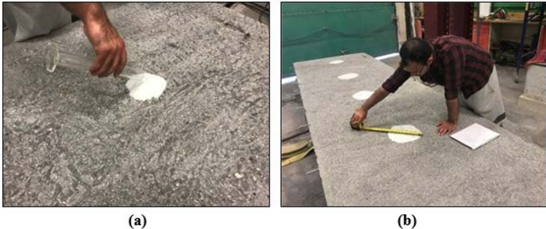
Figure 19. (a) Textured girder substrate and (b) determination of texture depth.
