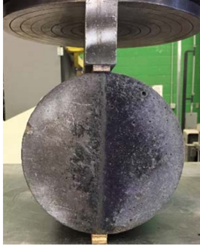
Figure 5. Split cylinder test setup.
