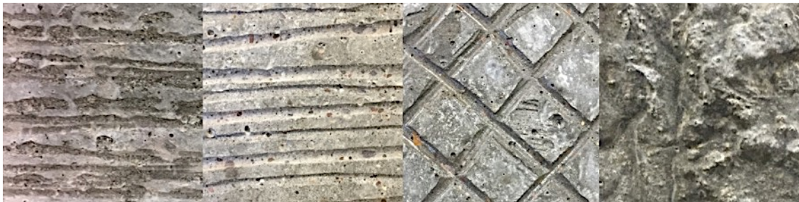
Figure 3. Surface texturing on substrate specimens, 0.002 in. (0.05 mm), 0.035 in. (0.9 mm), 0.063 in. (1.6 mm), and 0.11 in. (2.8 mm), from left to right, respectively.
