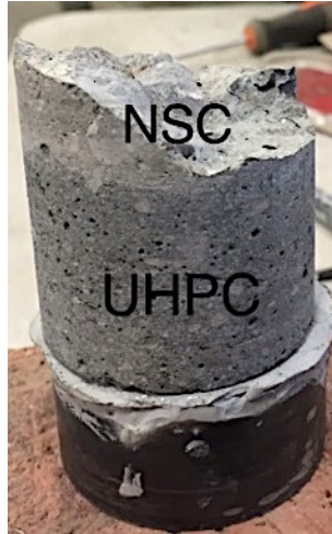
Figure 32. Substrate failure in direct tension specimen.
