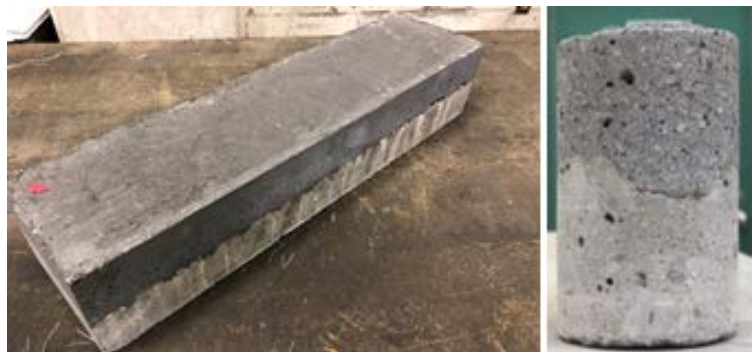
Figure 7. Direct tension specimens.
