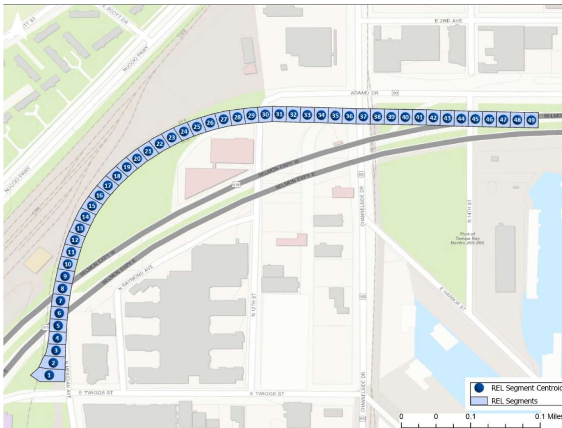
Figure 14. Map. Segmentation of the REL for Measuring Queue Lengths in Use Case 1
