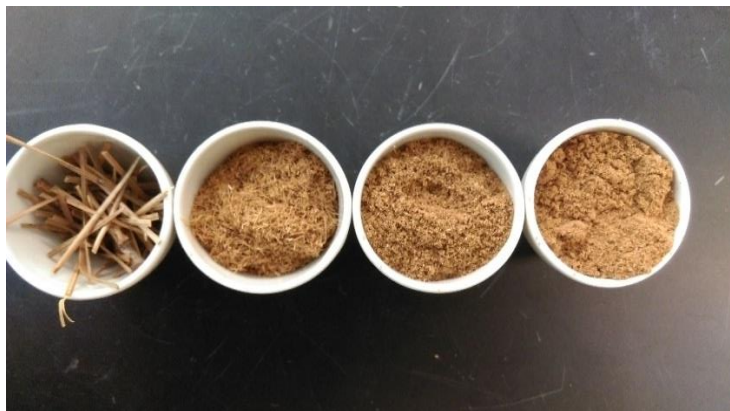
Fig. 1 Pine needles grinded to mesh size 10 – 35, 35 – 60 and > 60 microns
