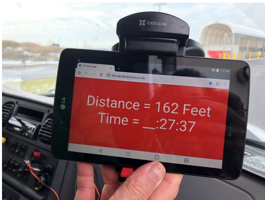
Figure 31. Following Distance < Target Distance (172 ft) Screen.
