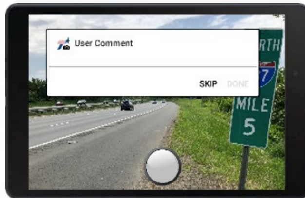
Figure 7.4 The user interface of the Android application to collect on-demand road conditions images
