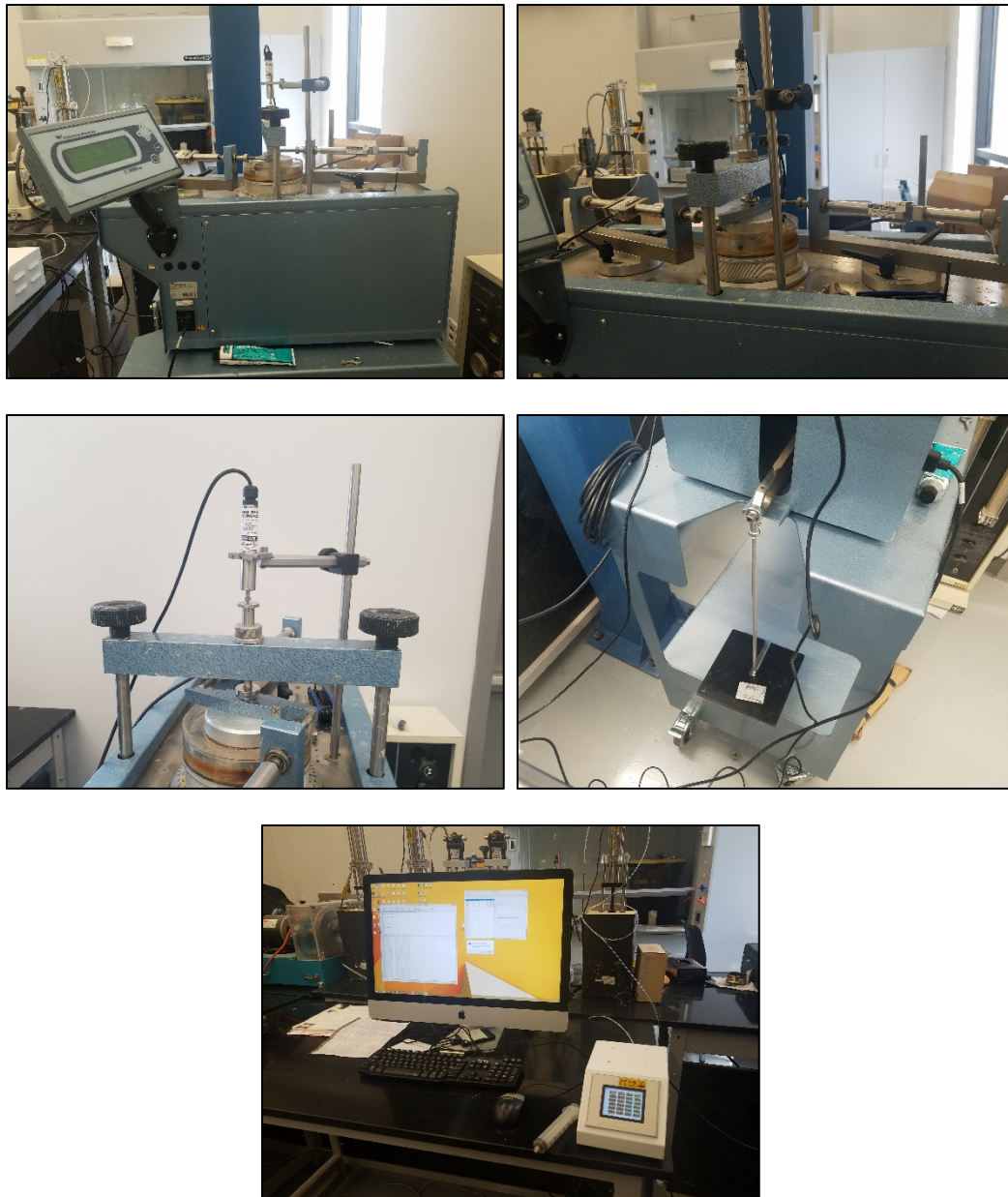
Figure 13. Components of the ring shear device test setup.
