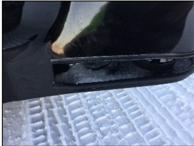
Figure 3-16 Snow Accumulation in Sensor Housing
