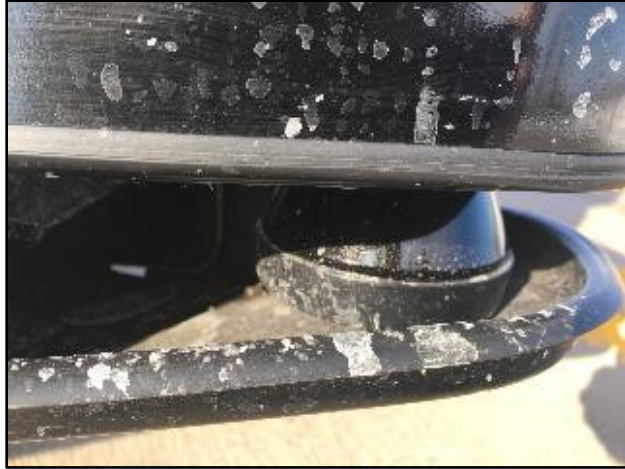
Figure 3-15 Road Salt on LIDAR Sensor
