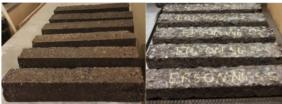
Figure 4.12. Original CIR beams and cut test beams.
