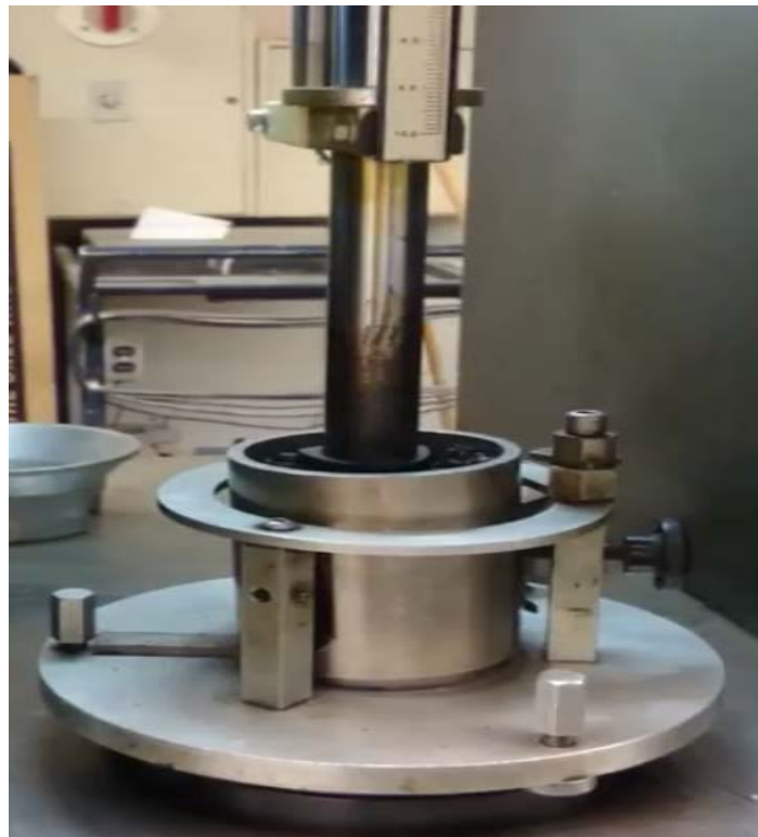
Figure 3.3. Hveem kneading compaction set-up.
