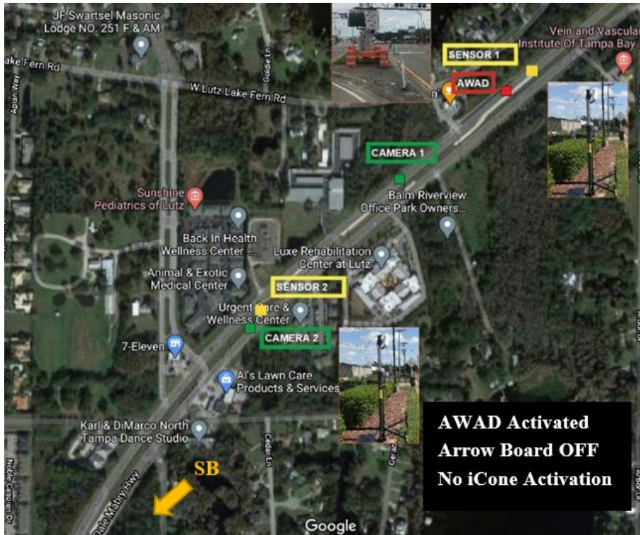
Figure 74. Layout of Data Collection for AWAD Scenario on N Dale Mabry Hwy
