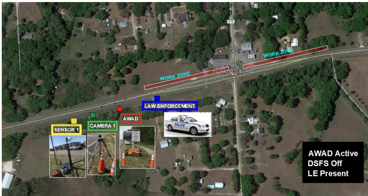
Figure 48. Deployment of “After 2/AWAD+LE” for Phase 4B2 at US-98 and Trilby Rd
