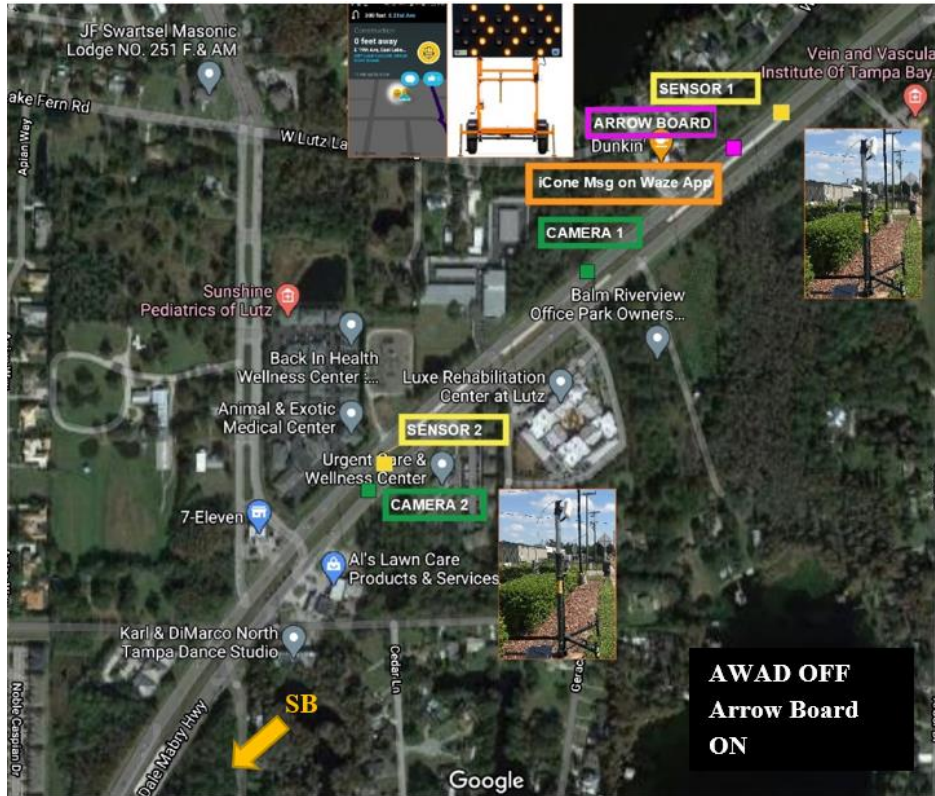
Figure 76. Layout of Data Collection for Arrow Board + iCone on N Dale Mabry Hwy
