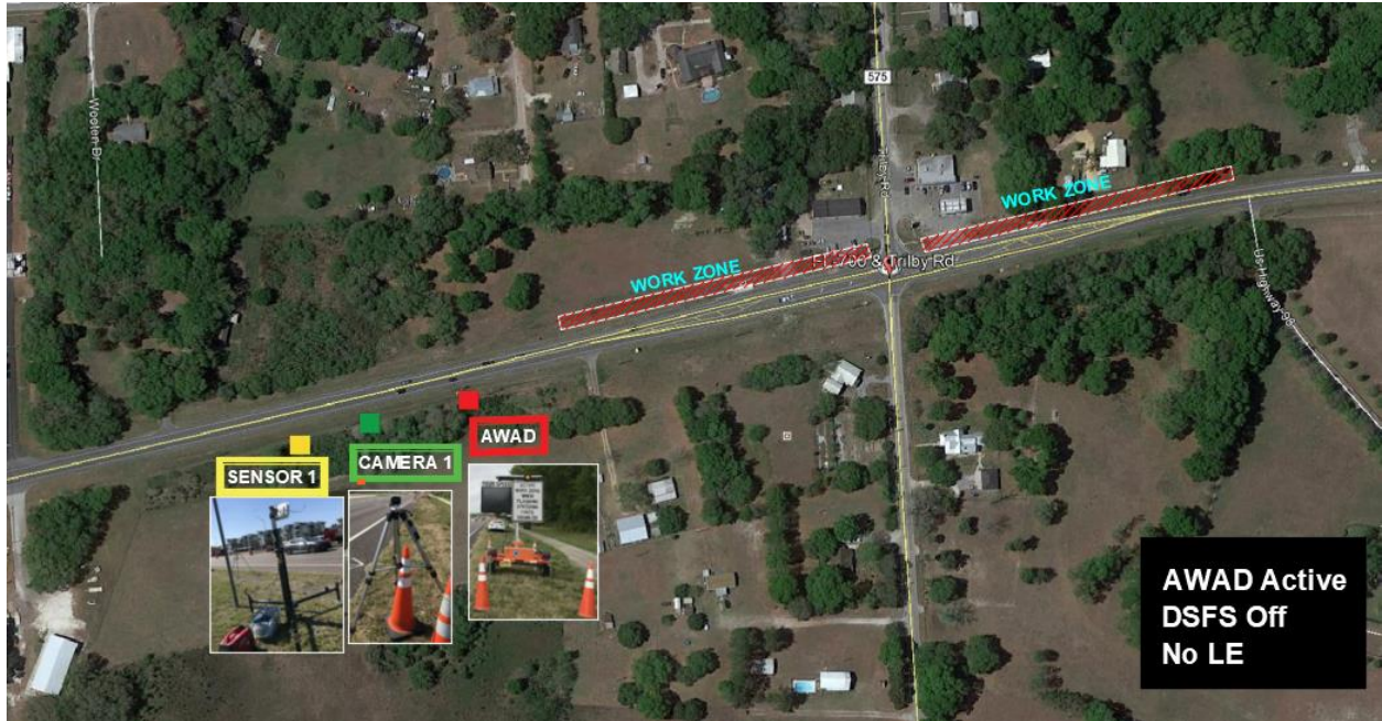
Figure 47. Deployment Stage of “After 1/AWAD” for Phase 4B2 at US-98 and Trilby Rd
